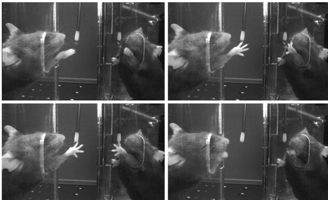
Figure 4.1: Samples of video frames illustrating the different phases of a reach-to-grasp movement collected during the early-prototype experiment.
