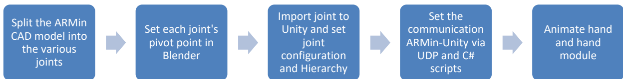
Figure 3.10 - ARMin's digital twin development workflow.
