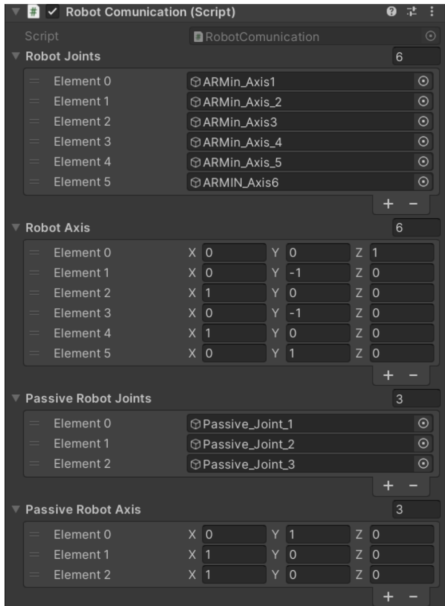
Figure 3.9 - Assigned components of the Robot Communication script, used to get joint's data from ARMin and translate it to the VE. Each joint was assigned the movement/rotation axis, as well as the direction, with a "-" representing the counterclockwise direction.
