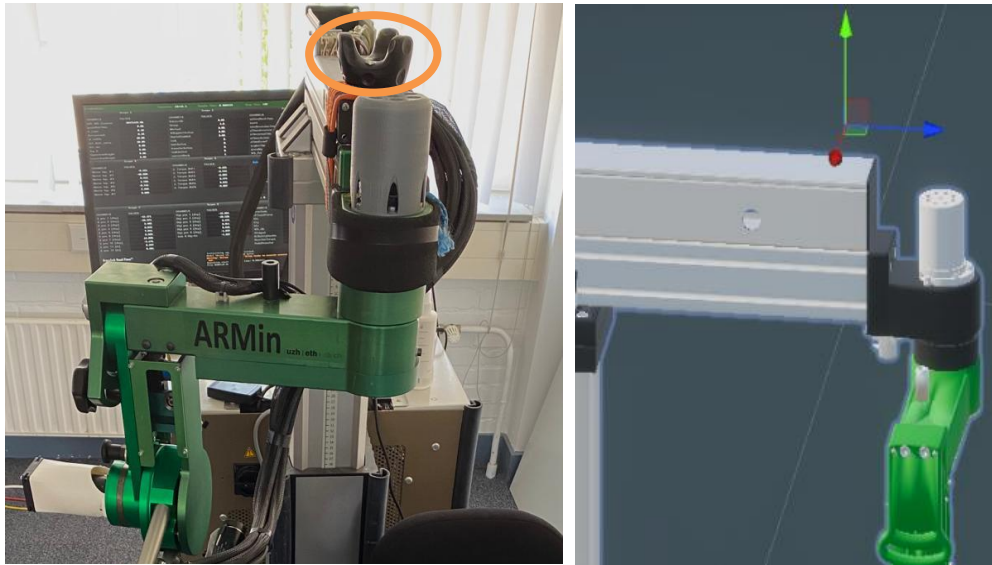
Figure 3.12 - Positioning a tracker on top of ARMin and its reference point in the VE. Upon starting the simulation, the position of the tracker would be recorded on the VE, from which the reference point would move to that position and subsequently the entire ARMin, thus being at the same location as the real robot.
