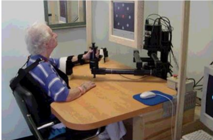
Figure 2.2 - MIT-Manus's end-effector rehabilitation robot from Interactive Motion Technologies, Cambridge, MA. Figure taken from [55].
