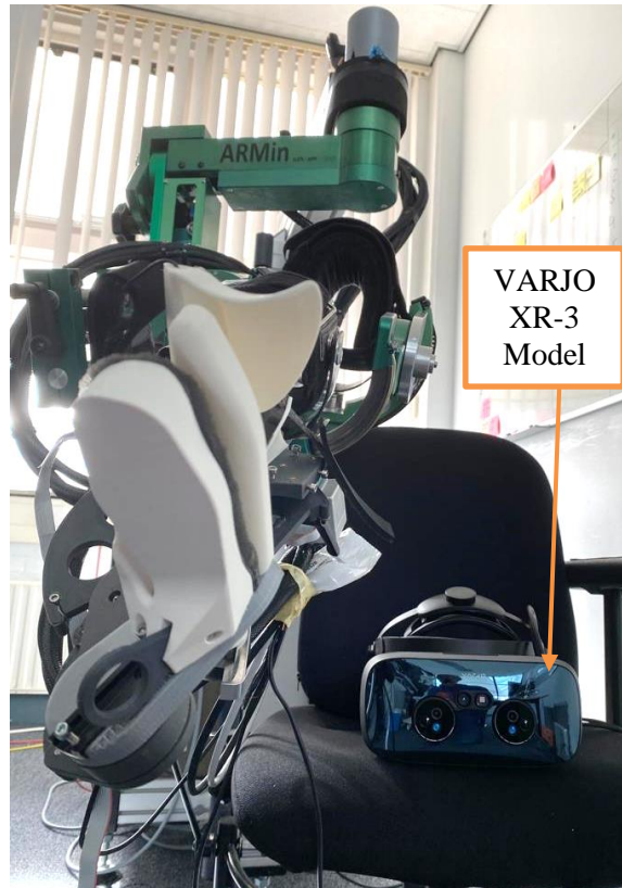
Figure 3.11 - ARMin upper limb rehabilitation robot with PRIDE hand module and Varjo XR-3 HMD.
