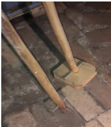
Figure 14: Cap punch down tools, right- applied in case of white wines; left- applied in case of red wines at Bolero & Co
