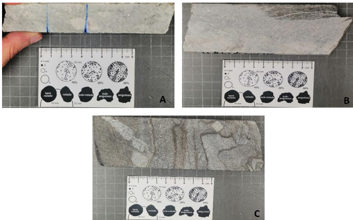
Figure 4.1 Examples of the different domains found in the studied drill hole. A) Macroscopic sample of aplite-pegmatite domain; B) Macroscopic sample of metasomatic alteration zone domain; C) Macroscopic sample of the host rock.
