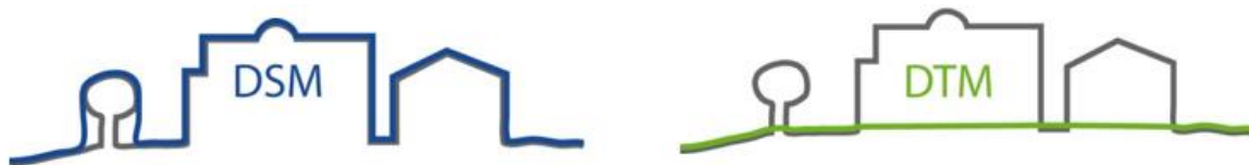
Figure 2.6 - Differences between DSM (surface model that includes structures and vegetation) and DTM (terrain model, represents relief at ground level) [Source: https://3dmetrca.it/ ]
