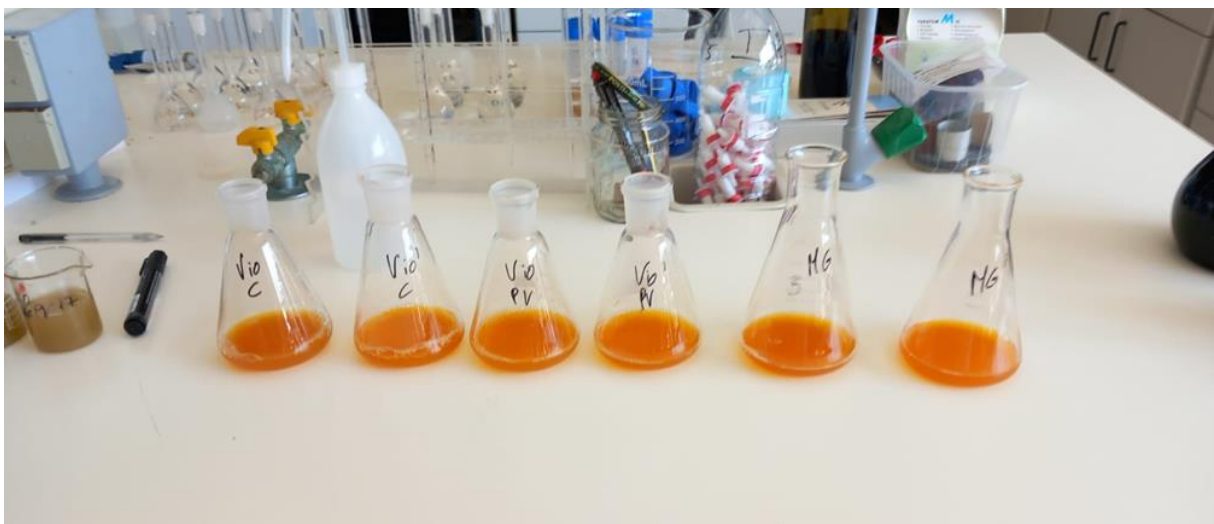
Figure 12: Image of the laboratory procedure analysis, particularly the solution of must and reagents in order to analyse the total acidity. In the pictures are presented the Viosinho samples, divided in PV and control along with other varieties s which were being analysed at that time.
