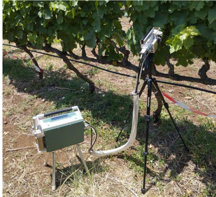
Figure 10 Illustration of the IRGA Li-6400 used for the data collection, with the tripod to fix the camera for the evaluations.
