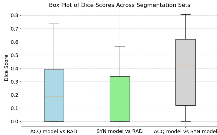
Figure 4.7: Boxplots of the distribution of Dice similarity coefficients for lesion segmentation performance on the PROSTATEx validation set. The plots compare the radiologist-defined ground truth (RAD) versus the ACQ model, RAD versus the SYN model, and the ACQ model versus the SYN model.
