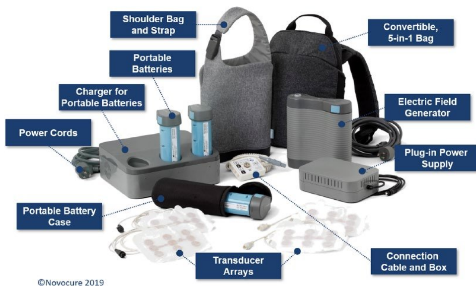
Figure 1.4: Components of the Optune™ device. The electric field generator can be powered by portable batteries, which can last between two to three hours, or by plugging it into a socket. The generator is connected to four arrays with 9 transducers each that work in pairs. These arrays are placed on the patient's shaved scalp in specific regions to induce the highest EF possible in two perpendicular directions alternately. Image taken from [30].
