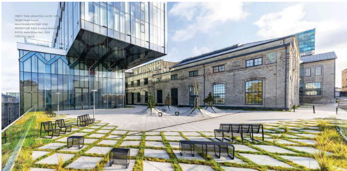
Figure 27. Fahle outdoor space, KINO Landscape Architects. The narrow strips of soil between the tiles also give plants enough growth opportunities, and the overall impression of the rocky surface is green. Photo: Terje Ugandi
