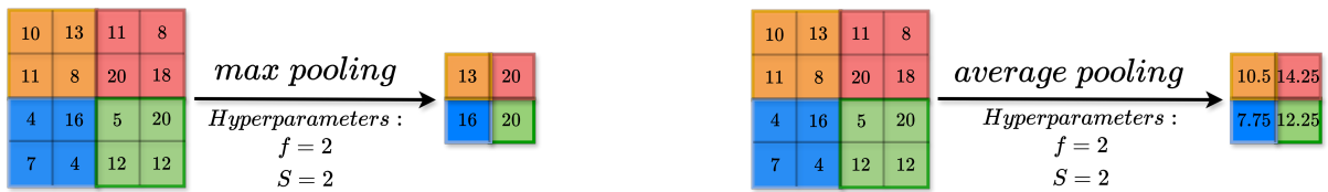
Figure 3.8: This illustration demonstrates the reduction of feature map dimensions following the application of max pooling, on the left side, and of average pooling, on the right side. For these instances, a 2 \times 2 kernel with a stride of 2 was employed. The colour scheme represents the kernel's positions on the input matrix and their corresponding outputs in the feature map.
