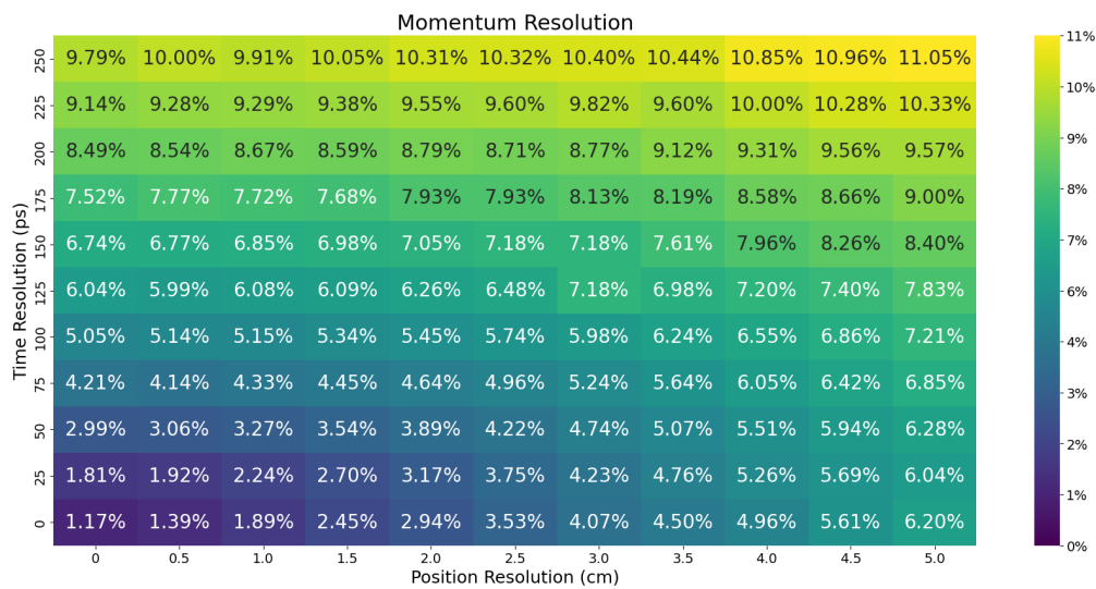
Figure 4.15: Comparison of momentum resolutions for protons particles at 500 MeV/u, considering different values of position and time resolutions.
