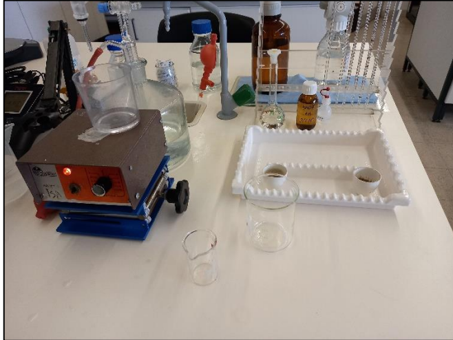
Fig 11. Laboratorial assembly for acid-base titration and pHmeter.
