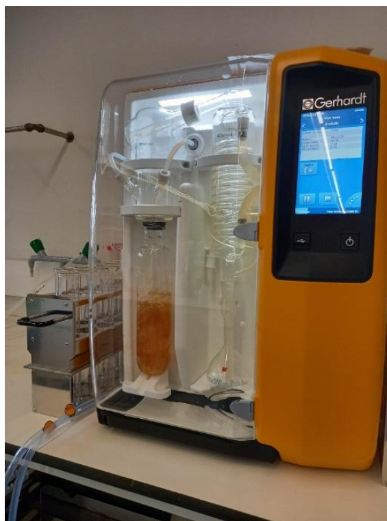
Fig 10. Automatic Distiller at the Laboratory of Enology, Instituto Superior de Agronomia.
