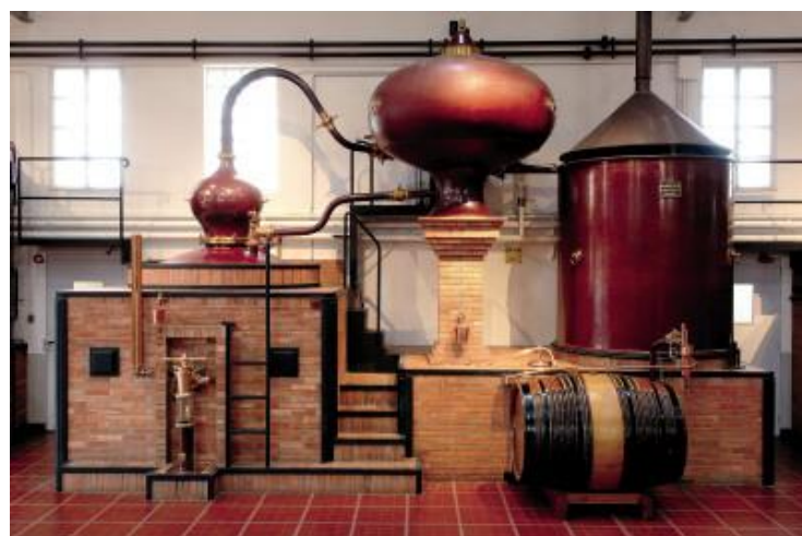
Fig 2. Discontinuous Alembic Still. Source: https://cognacecotognata.wordpress.com/2012/01/27/cognac-la-distillazione-lalambicco-1-parte/
