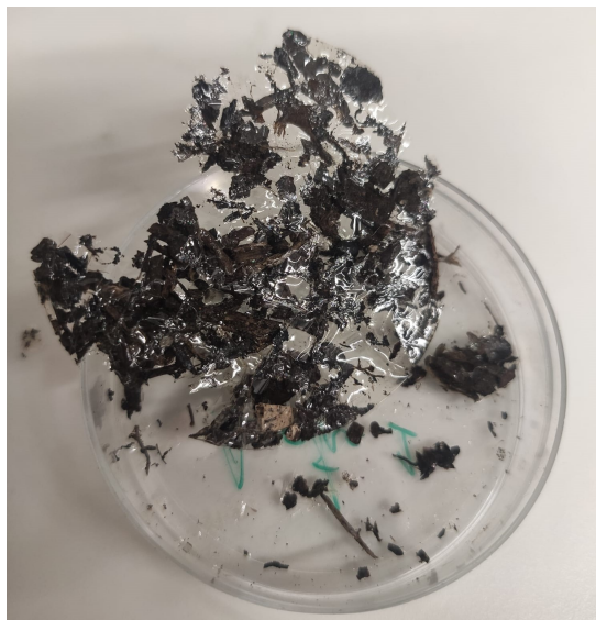
Figure 4.30: Preliminary biodegradability tests showed visible hydrogel adhesion to the soil. This result prevented the measurement of the hydrogels biodegradability over a period of three weeks.
