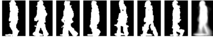
Figure 3.2: Example of GEI robustness in the presence of shadows in the corresponding silhouettes [52].
