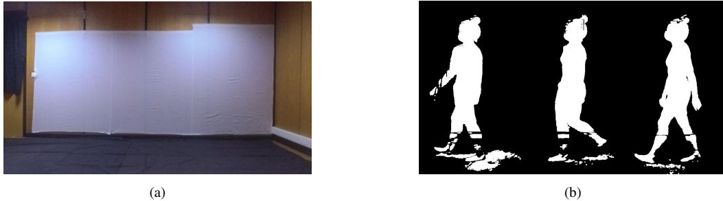
Figure 4.4: Background subtraction results on the second setup. a) Setup; b) Main errors of background subtraction;
