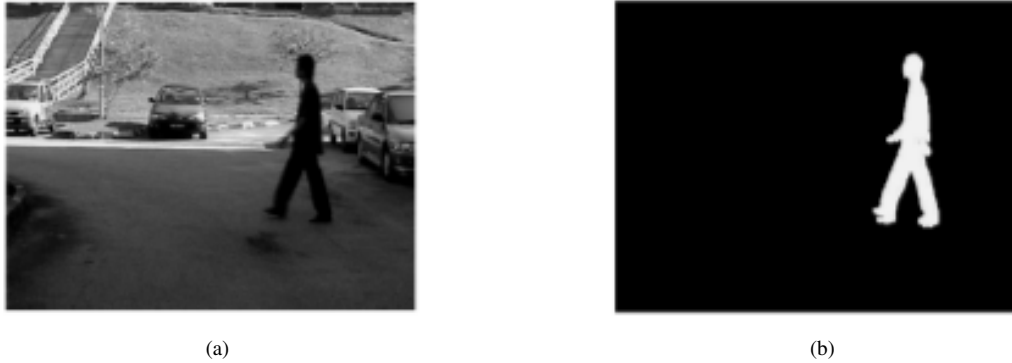
Figure 3.1: Example of background subtraction [50]. a) Original frame; b) Corresponding foreground mask after subtracting the background.
