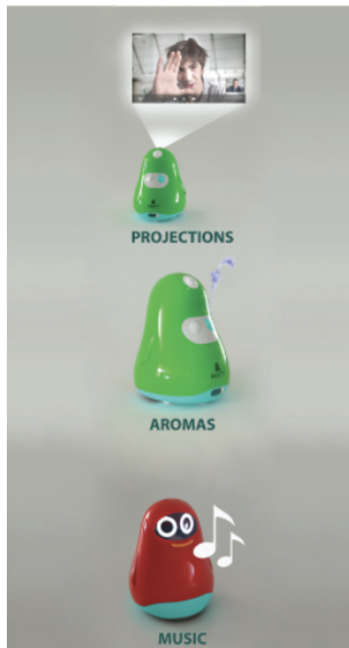
Figure 2.3: MATY v4: the last prototype materialized expressing examples of the multisensorial service provided to elicit the person with Alzheimer through the day[165].
