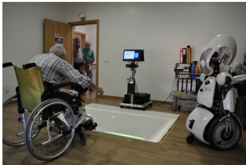
Figure 2.5: Vizzy a wheeled humanoid robot, used as an exercise coach, explaining the activity to the participant [13].
