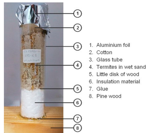
Figure 2. Termite attack test assembling, with, in this example, EPS-S as the insulation material and the termite species Reticulitermes grassei , after 24 h of exposure.
