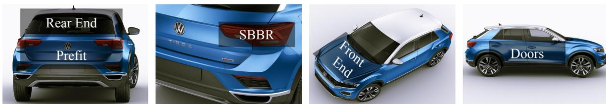
Figure 4.1: Volkswagen model with shadows above the car parts to be aligned in each fitting process type.
