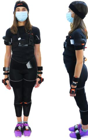
Figure 4.2: Inertial Motion Capture systems setup. MVN Awinda and Fraunhofer's systems that consisted of 17 and 7/8 Inertial Measurement Units, respectively. Representation of standing in the N-Pose.
