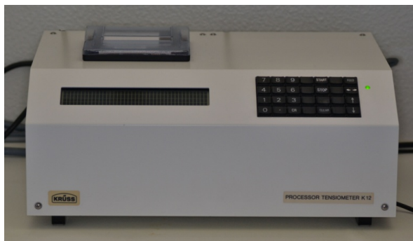
Figure 10 and 11 – Processor Tensiometer K12 (Kruss, Hamburg, Germany): equipment used in Wilhelmy plaque technique.
