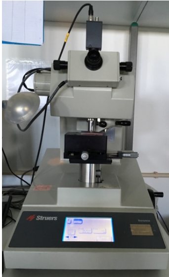
Figure 7 – Microhardness indentation machine (Duramin, Struers DK 2750, Ballerup, Denmark).
