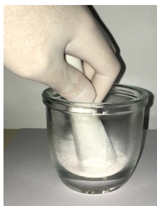
Figure 4.3 – Homogenization of chlorhexidine in the powder of the reline acrylic resin, using a mortar and pestle.
