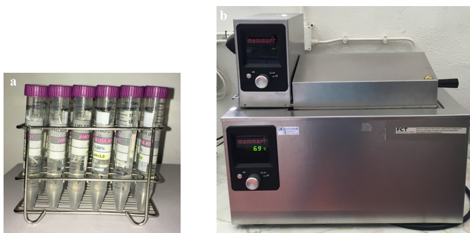
Figure 5.2 – Chemical aging protocol. a) Incubation of the specimens in graduated falcon tubes with artificial saliva; b) Incubator (Mettmert, Schwabach, Germany).
