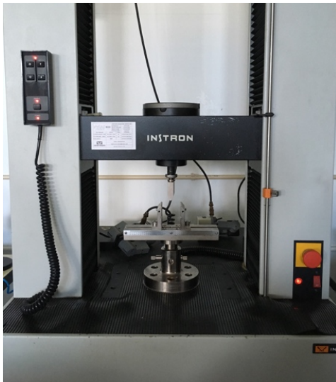
Figure 8 – Servo-hydraulic testing machine (Instron model 4502, Instron Ltd, Bucks, England).
