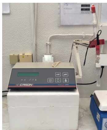
Figure 19 – pH meter (Crison Micro pH 2001, Hach Lange, Barcelona, Spain) used to prepare artificial saliva.
