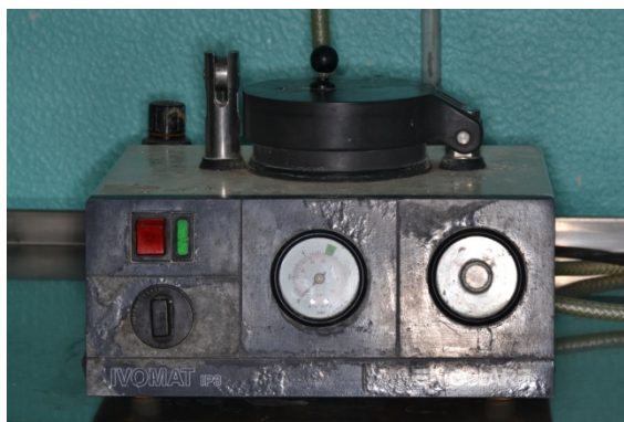
Figure 4.5 – Pressure device (Ivomat, Ivoclar Vivadent, Liechtenstein).
