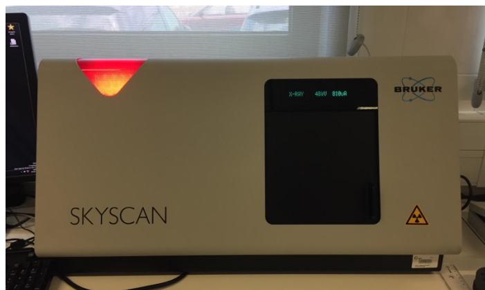
Figure 4.16 – Micro-CT device (SkyScan 1174; Bruker, Brussel, Belgium).
