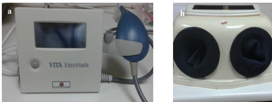
Figure 5.4 – Color measurement of the specimens. a) VITA Easyshade (ES) spectrophotometer; b) Dark chamber.
