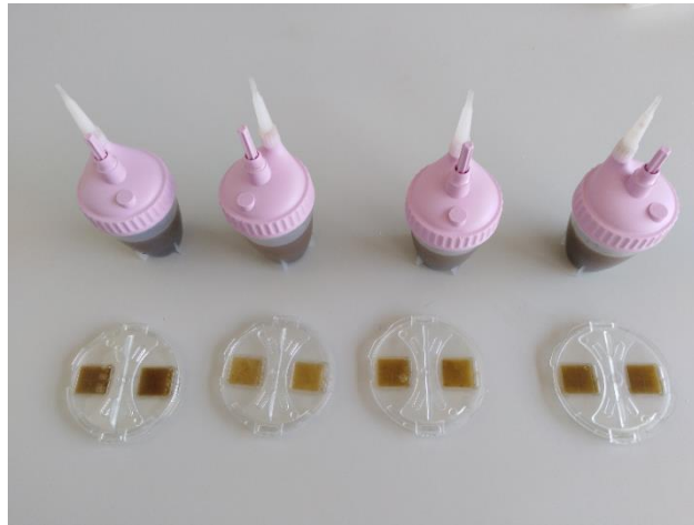
Figure 11. Mini-FLOTAC and Fill-FLOTAC devices used for quantitative coprology (original).
