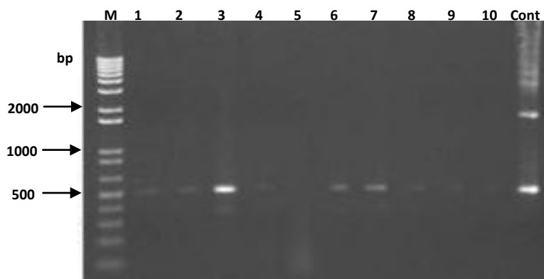
Figure 12: Agarose gel electrophoresis (1 % agarose, 5 µg/mL gel red) of the PCR amplification of the BLAD gene (~530 bp) using BLAD att primers and as template DNA extracted from the putatively transformed cell lines. Lane 1 – cell line 1 Glad tidings (GT 1); Lane 2 – cell line 12 Glad tidings (GT 12); Lane 3 – cell line 13 Glad tidings (GT 13); Lane 4 – cell line 18 Glad tidings (GT 18); Lane 5 – cell line 19 Glad tidings (GT 19); Lane 6 – cell line 3 Only love (OL 3); Lane 7 – cell line 4 (OL 4); Lane 8 – cell line 8 (OL 8); Lane 9 – cell line 14 (OL 14); Lane 10 – cell line 3 Tineke (T3); Lane M – marker 1 kb ladder (Invitrogen).
