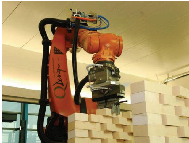
Fig. 20. Robot Bricklayer a colocar tijolos; empresa Gramazio & Kohler ( www.electronicsonline.com/News/New_Gadgets/Robotics/robot-bricklayer-builds-winery-with-precision.html ).
