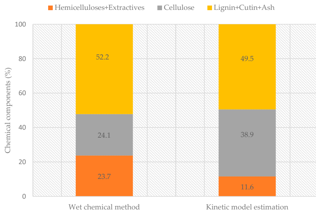
Figure 3. Comparison of chemical pine nutshell components (on a dry basis) determined by wet chemical analysis and estimated by kinetic modeling of thermogravimetric analysis.
