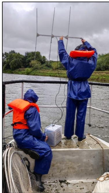
Figure I.6- Images of the manual active radio tracking procedure, by boat, using a manual radio tracking receiver (model R410) and a 4-element Yagi antenna, both from Advanced Telemetry Systems.
