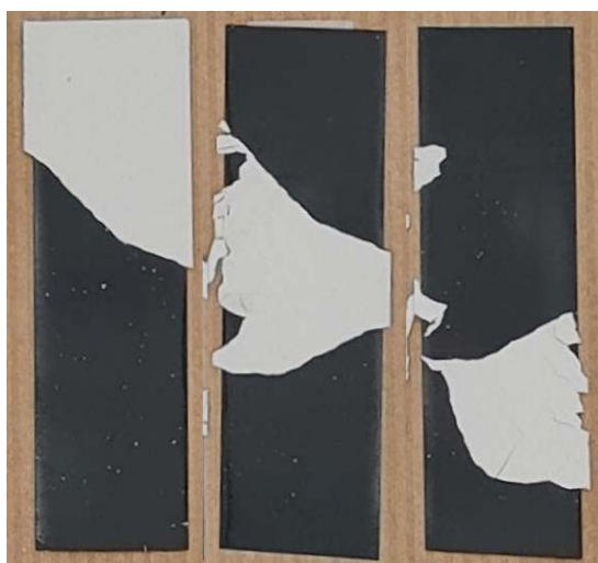
Fig. 7. Peeling test, filler detachment, an example of a specimen with Polyfilla only.
