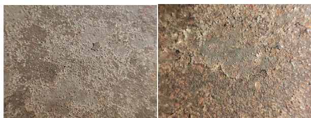
Fig. 2. The reverse side of the painting shows intricate details, including the presence of multicoloured iron corrosion products and residual traces of tin.
