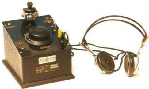
Fig 10. Galena radio receptor. @Museo Telecom UPV
