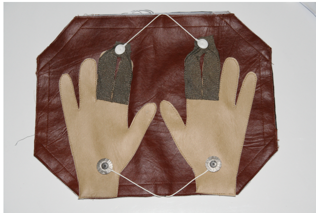
Figure 4.2: Electrocardiography sensors and electrodes arrangement. At the top: the electrolycra strips; At the bottom: the dry Ag/AgCl electrodes [2].
