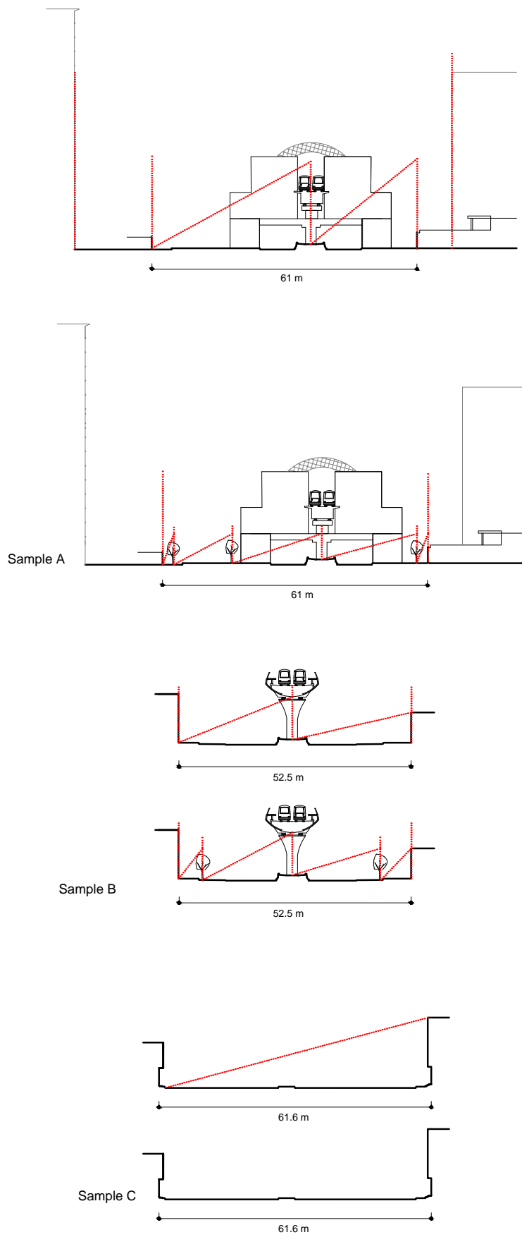
Figure 9.2-19 Abi Jafar Al Mansour Street: Cross-sections of samples "A, B, and C" show the street width and building height ratios. (Source: Author's Edition).
