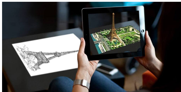
Figure 2.4: Example of marker-based tracking, Source: [60]
