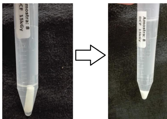
Figure 17 –a) Scaffold emerged in PBS before the shaking. b) Scaffold destroyed after the centrifugation.
