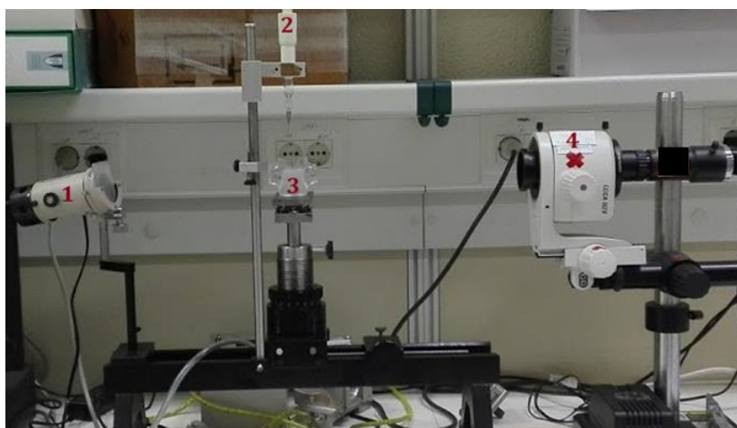
Figure 25 – Goniometer: 1) Light source 2) Micrometer syringe 3) Liquid cell 4) Video camera.
