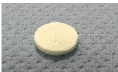
Figure 26 - Scaffold dried used in swelling assay.
