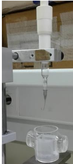
Figure 24 - Micrometer syringe with a needle inverted in the edge and the liquid cell.
