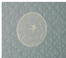
Figure 28 – Example of KBr tablet with scaffold powder blend.
