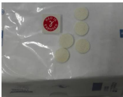
Figure 14 - Example of irradiated scaffolds. These were inserted in Tyvek bags with yellow gamma indicator and sent to Aragogamma. After the radiation, the indicator gets red, as a sign that the radiation occurred.
