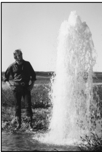
Figure 15 – Drill-hole flow from a pingo studied in 1976, on behalf of Mackay (1979). The gusher that rose to a maximum of 2.6 m issued from a 7.5 cm diameter hole with a depth of 22 m. The water temperature was about -0.1^{\circ}\text{C} . Source: Mackay (1998).
