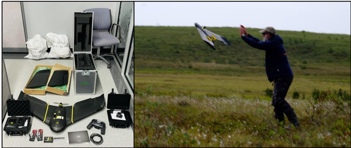
Figure 45 - SenseFly ebee Plus RTK UAV model (Left), and its launch at PCL on behalf of the July 2019 field campaign of CEG/IGOT - University of Lisbon and the Geological Survey of Canada (Right). Source: Canada DroneTrader (2021) (Left); Photo by Vieira (2019) (Right).
