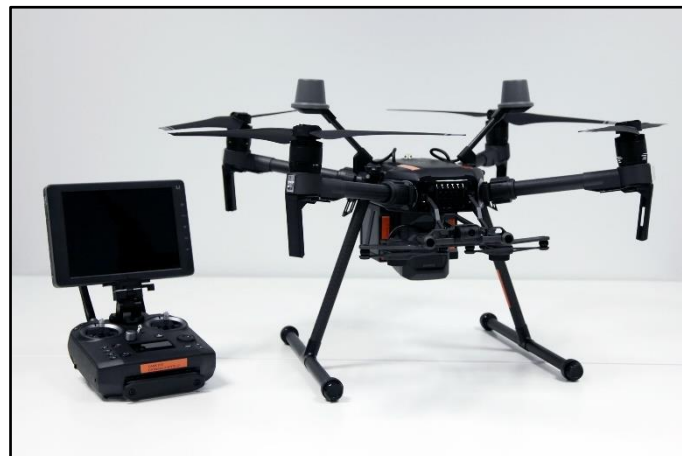
Figure 47 - DJI Matrice 210 RTK UAV model. Source: Arctic Drone Labs (2020).
