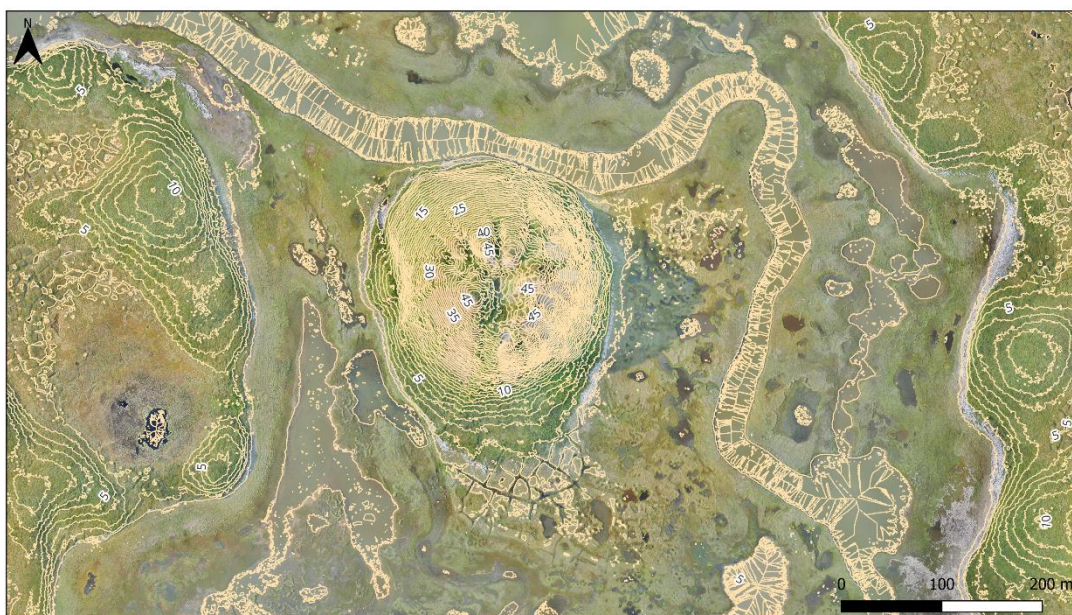
Figure 51 – Contour line map (1 m equidistance, with labels every 5 m), used as an aid in the elaboration of the Geomorphological Map. The view is the same as Figure 50.
