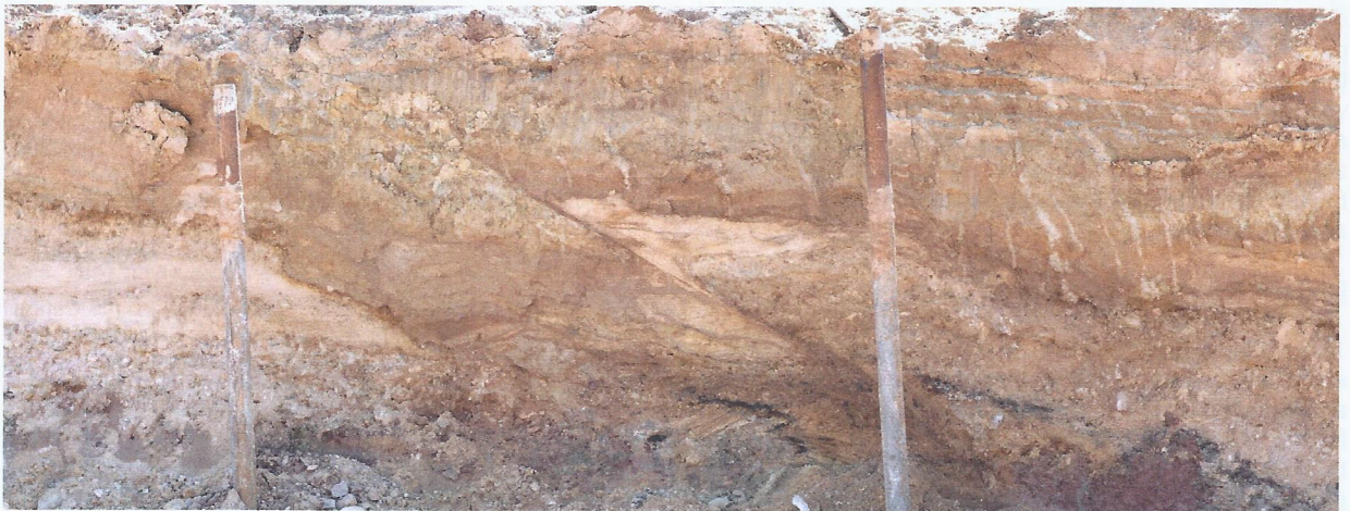
Figure 4: Reverse fault in Middle Pleistocene fluvial deposits that roots in Formação da Dagorda marls, at the same site.
