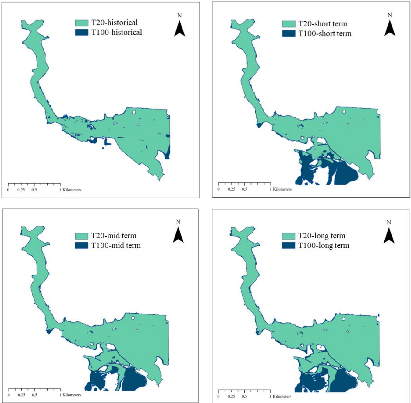
Figure 5.20: Flood extent maps for the two past flood events (historical) and the future flood scenarios (short, mid, and long term development).
