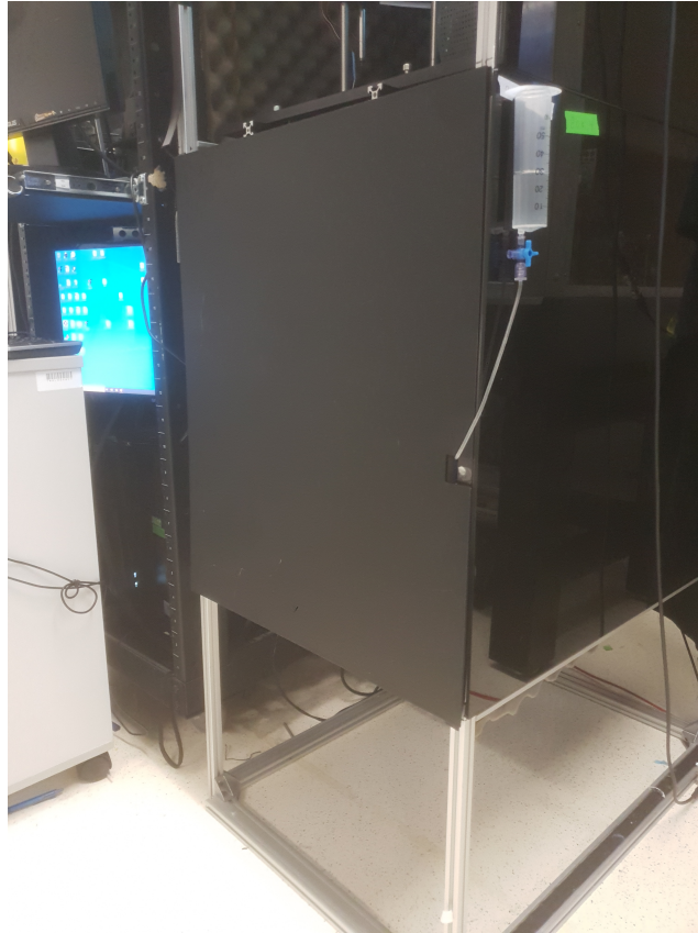
Figure 7: A closed training box. The acrylic doors are magnetically mounted on the frame of the enclosure assembly.
