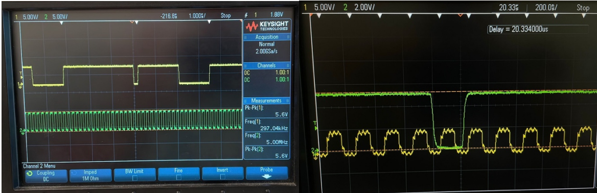
Figure 3.19 - On the left, the green wave represents the enable signal ranging from 0 (low) – 5 V (high) and the yellow wave represents the output enable signal, where it is possible to identify two complete intervals where the measuring wasn't being done (0 V) and a complete interval of 5 V (measuring range interval) where one pulse had been removed (0 V inside of the measuring range interval); On the right, the green wave represents the output enable signal and the yellow wave was the signal that came from the PCB. It is also possible to see that the interval of removing a wave matched with a complete pulse of the yellow wave.
