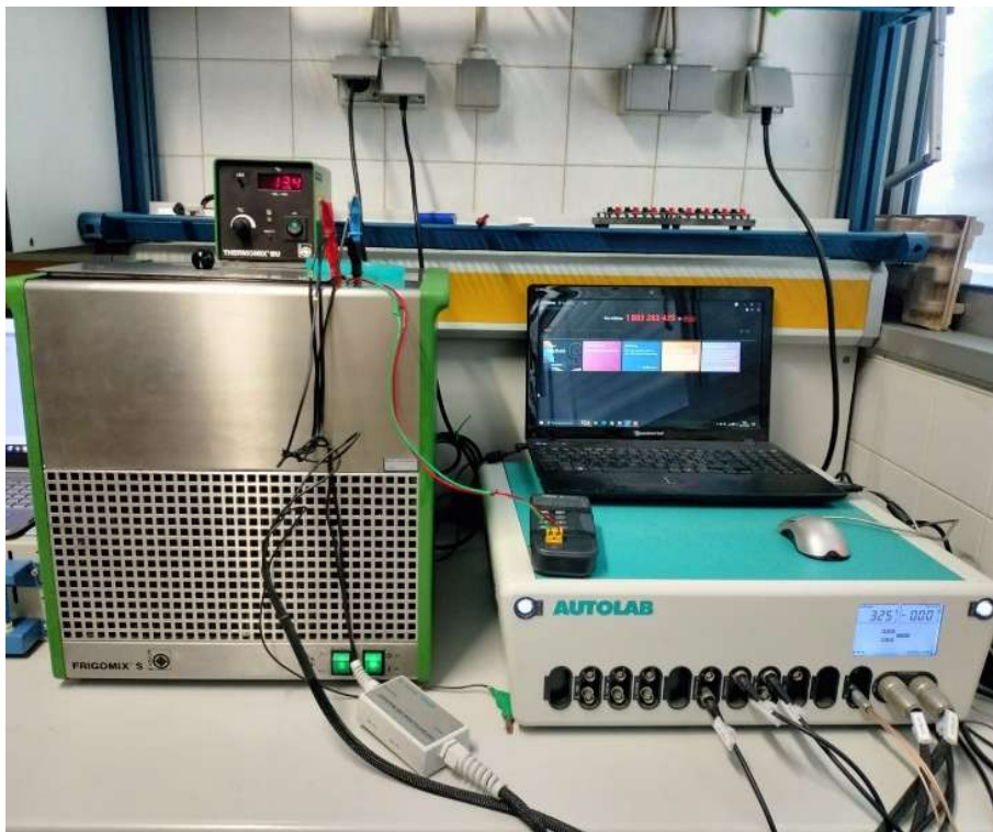
Figure A.2.4: Integration of the EIS Autolab equipment with the cryostat. On top of the Autolab device, a laptop equipped with control software and a thermocouple oil sensor is placed.
