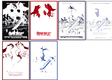
IMAGE CLUSTER PARTITIONS Pixels of the image assigned to each cluster. The border is the color of the cluster as calculated by the average value of its pixels.
