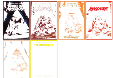
IMAGE CLUSTER PARTITIONS Pixels of the image assigned to each cluster. The border is the color of the cluster as calculated by the average value of its pixels.
