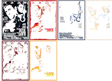
IMAGE CLUSTER PARTITIONS Pixels of the image assigned to each cluster. The border is the color of the cluster as calculated by the average value of its pixels.
