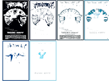
MAGIC CLUSTER PARTITIONS Pixels of the image assigned to each cluster. The border is the color of the cluster as calculated by the average value of its pixels.
