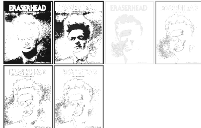
IMAGE CLUSTER PARTITIONS Pixels of the image assigned to each cluster. The border is the color of the cluster as calculated by the average value of its pixels.
