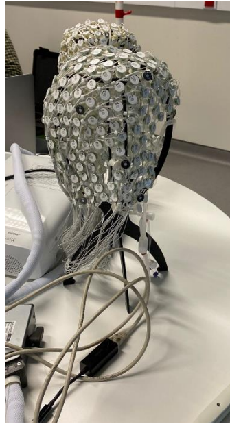
Figure 4.4: EEG cap used for the experiment. Developed by Magtism EGI.
