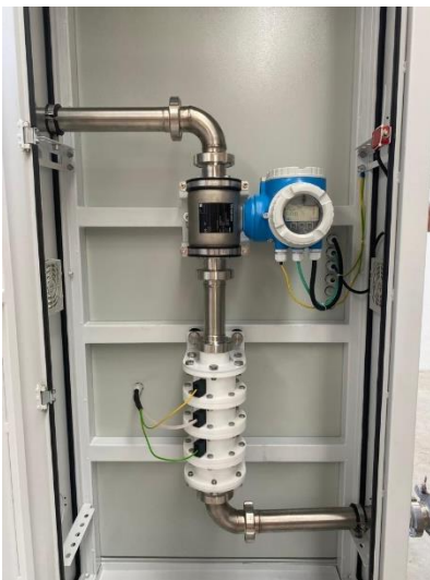
Figure 3.2 Co-linear PEF treatment chamber used before pressing with vertical configuration.
