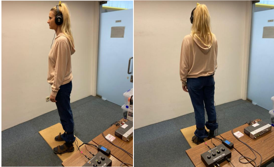
Figure 2.2: ‘Magic Shoes’ sound device, comprised of a pair of strap sandals, two microphones attached to the sandals, an M-track duo amplifier and a stereo 9-band graphic equalizer that amplifies the sounds and changes the sound spectra.
