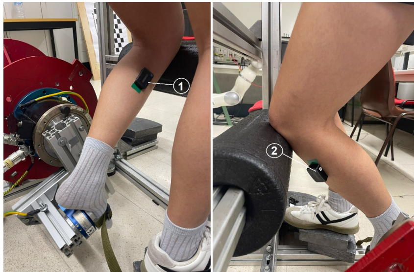
Figure 3.8: Electrodes muscle positioning: (1) Gastrocnemius electrode; (2) Tibialis Anterior electrode.
