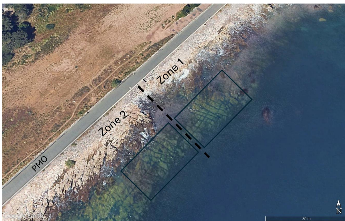
Figure 8.14 – Zones 1 and 2 separated by a black dashed line, where it is possible to observe that transitioning from Zone 1 to Zone 2, the fracture pattern becomes much more heterogeneous.
