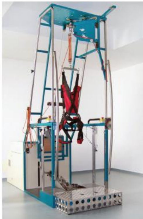
Figure 3.4 – Gait Trainer GT1 (picture courtesy of Reha-Stim). The patient is suspended in a harness from a wire above for body weight support. The subject's feet are placed on footplates that move in elliptical motions that simulate the different stages of one gait cycle. Figure removed from [12].
