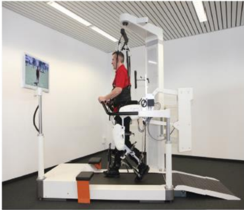
Figure 3.3 – Lokomat Pro version 6.0 (picture courtesy of Hocoma). This picture shows a person strapped in a Lokomat Pro version 6.0. The person is suspended in a harness from a wire above for body weight support and moved by attachments at the lower back to the robotic exoskeleton. The subject's legs are strapped in the exoskeleton which is actuated at the hip and knee. The forefoot is stepped upwards with a spring to induce dorsiflexion. Figure adapted from [12].
