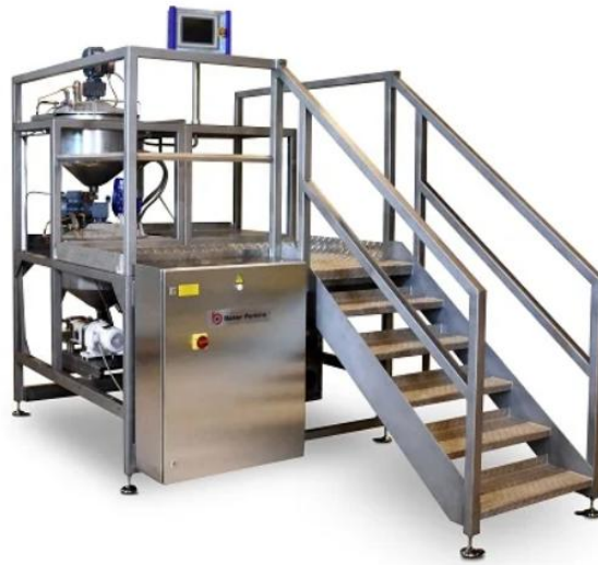
Figure 7 - JellyCook™ batch cooker. 50kg/hour ServoForm™ Mini depositor.
