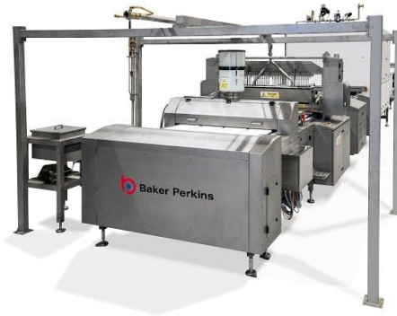
Figure 8 - Baker Perkins' ServoForm™ Jelly depositors (3D/2D). 1900 kg/h.
