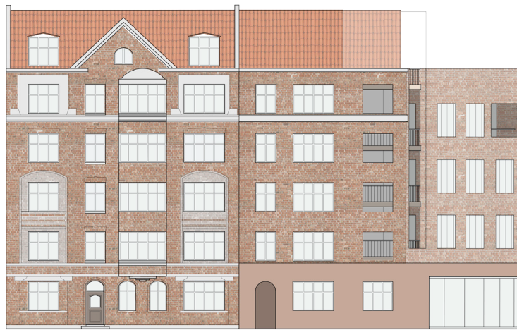
Ill. 59 – Alignment of the windows from Sundholmsvej 57 (left) and the cores of the proposal (right).
