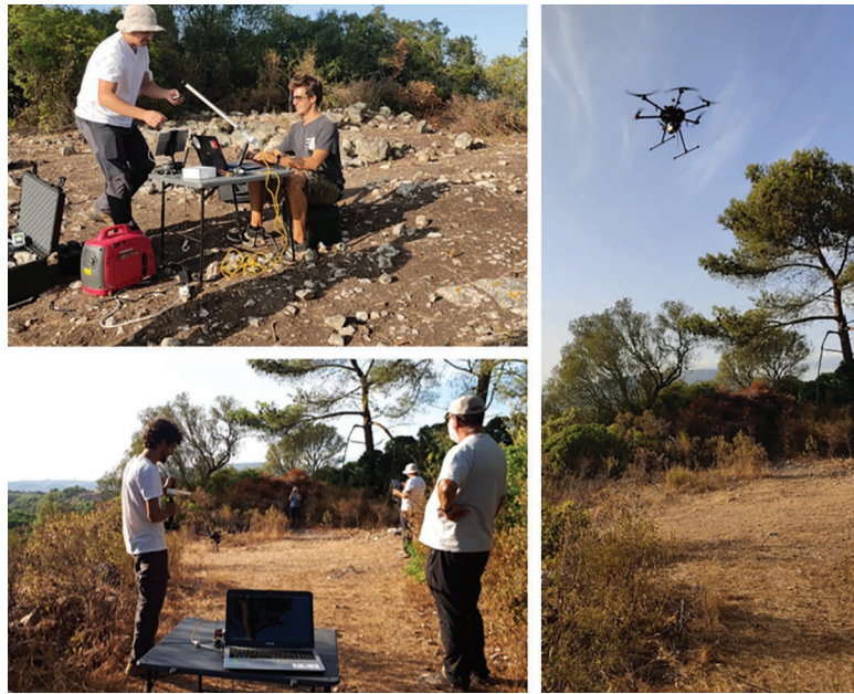
Fig. 3. LiDAR data acquisition system: a, b in-site base station; c Data acquisition with a DJI Matrice 600 Pro.
