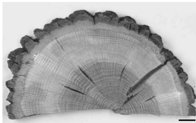
Figure 1. Stem cross-section of Quercus faginea showing the natural colour differences between heartwood and sapwood (bar = 2 cm).
