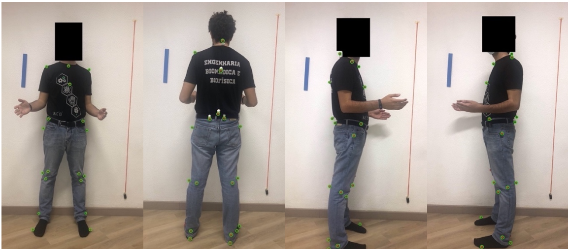
Figure B.33: Images captured with flash of the participant wearing a black shirt and jeans while using red styrofoam spheres as markers. The markers detected by the software are surrounded with green circles. On the left: Anterior view. In the middle left: Posterior view. In the middle right: Right lateral view. On the right: Left lateral view.
