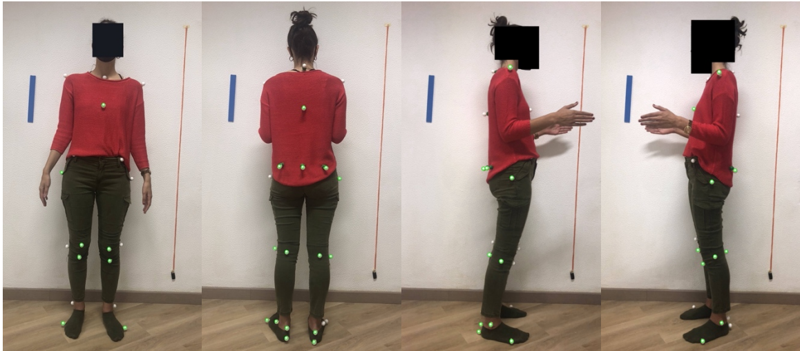
Figure B.15: Images captured with flash of the participant wearing a red shirt and green pants while using white styrofoam as markers. The markers detected by the software are surrounded with green circles. On the left: Anterior view. In the middle left: Posterior view. In the middle right: Right lateral view. On the right: Left lateral view.
