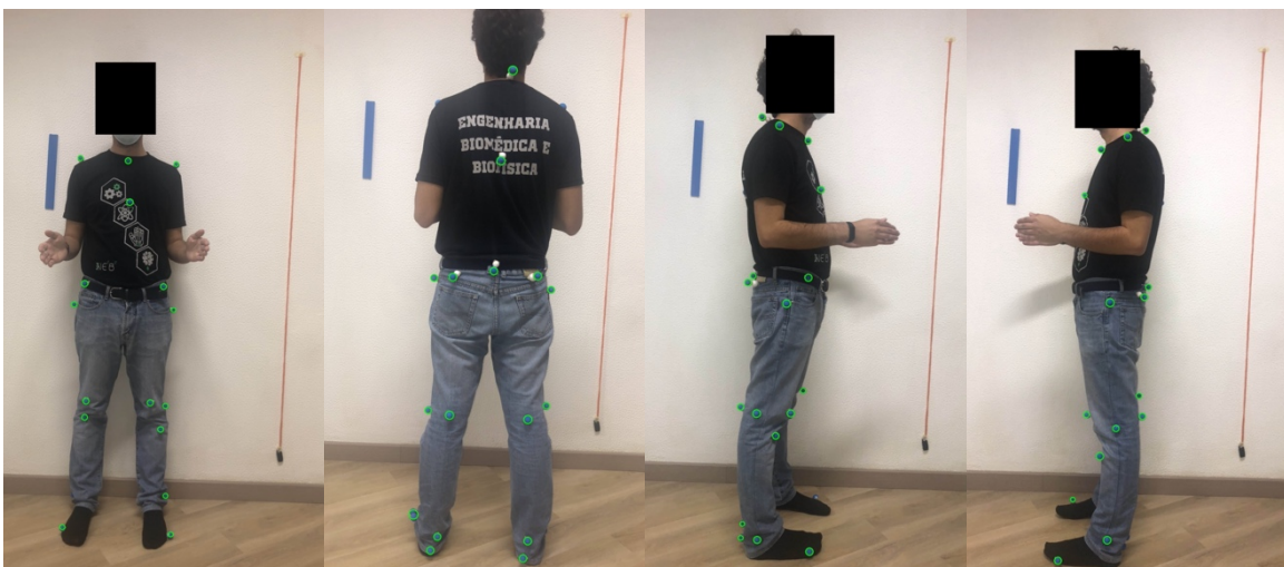
Figure B.41: Images captured with flash of the participant wearing a black shirt and jeans while using blue styrofoam spheres as markers. The markers detected by the software are surrounded with green circles. On the left: Anterior view. In the middle left: Posterior view. In the middle right: Right lateral view. On the right: Left lateral view.
