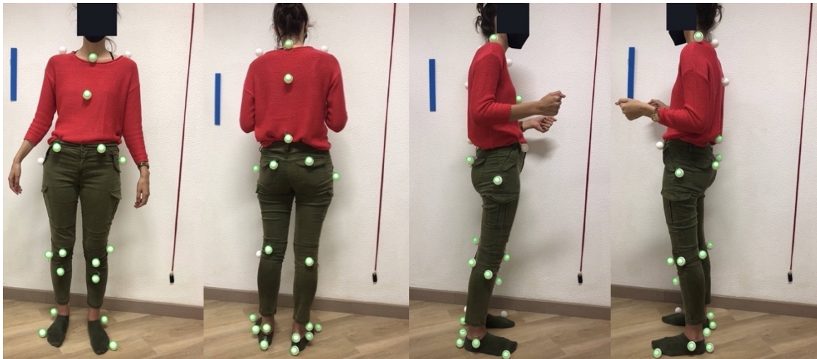
Figure B.7: Images captured with flash of the participant wearing a red shirt and green pants while using white ping pong balls as markers. The markers detected by the software are surrounded with green circles. On the left: Anterior view. In the middle left: Posterior view. In the middle right: Right lateral view. On the right: Left lateral view.
