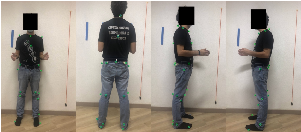
Figure B.42: Images captured without flash of the participant wearing a black shirt and jeans while using blue styrofoam spheres as markers. The markers detected by the software are surrounded with green circles. On the left: Anterior view. In the middle left: Posterior view. In the middle right: Right lateral view. On the right: Left lateral view.
