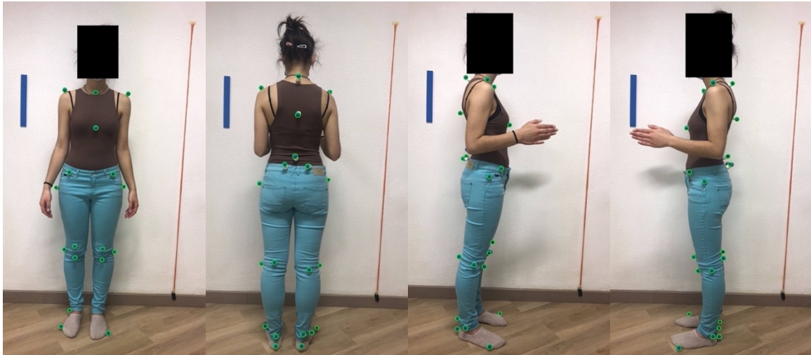
Figure B.45: Images captured with flash of the participant wearing a brown shirt and blue pants while using blue styrofoam spheres as markers. The markers detected by the software are surrounded with green circles. On the left: Anterior view. In the middle left: Posterior view. In the middle right: Right lateral view. On the right: Left lateral view.
