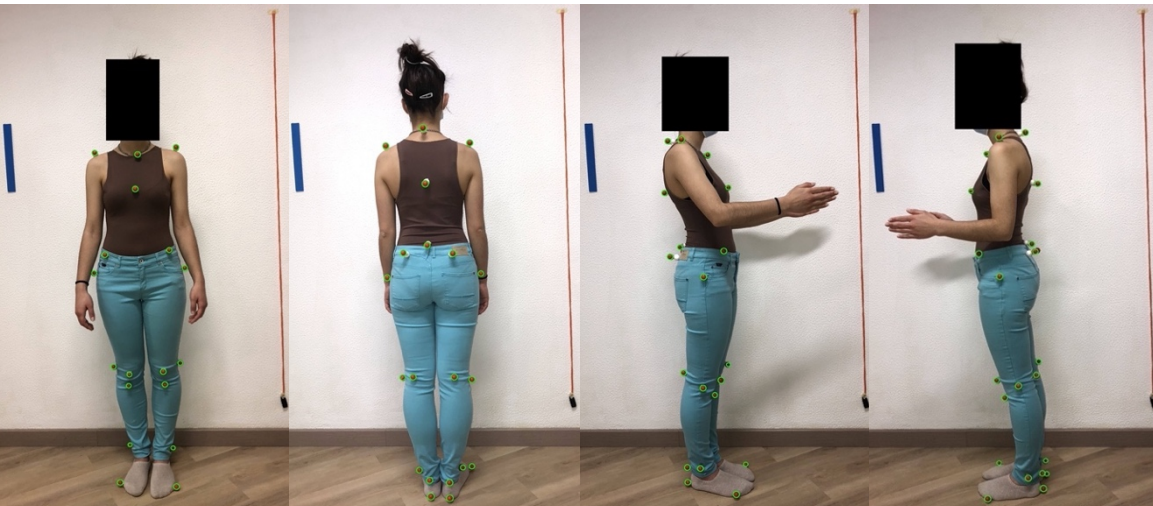
Figure B.37: Images captured with flash of the participant wearing a brown shirt and blue pants while using orange styrofoam spheres as markers. The markers detected by the software are surrounded with green circles. On the left: Anterior view. In the middle left: Posterior view. In the middle right: Right lateral view. On the right: Left lateral view.
