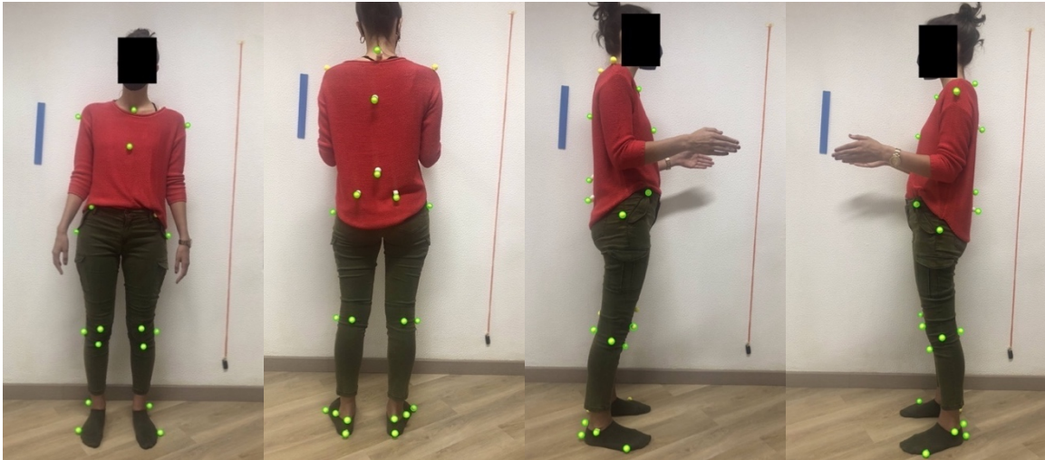
Figure B.24: Images captured without flash of the participant wearing a red shirt and green pants while using yellow styrofoam as markers. The markers detected by the software are surrounded with green circles. On the left: Anterior view. In the middle left: Posterior view. In the middle right: Right lateral view. On the right: Left lateral view.
