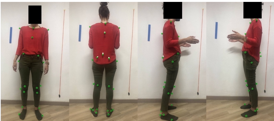
Figure B.56: Images captured without flash of the participant wearing a red shirt and green pants while using green styrofoam as markers. The markers detected by the software are surrounded with green circles. On the left: Anterior view. In the middle left: Posterior view. In the middle right: Right lateral view. On the right: Left lateral view.
