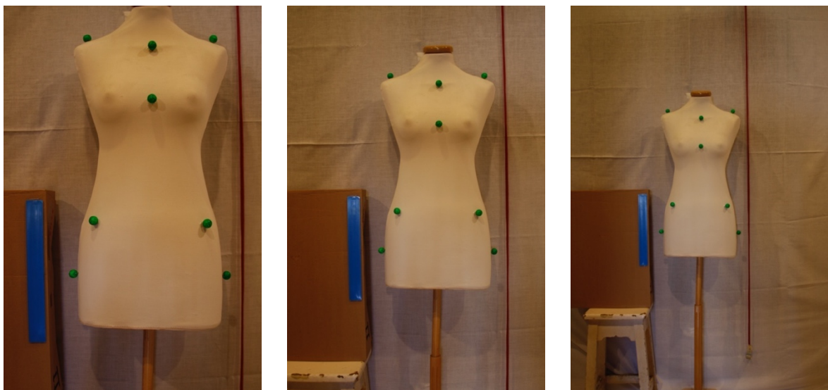
Figure C.12: Images captured without using flash with a photographic camera at a height of 100 cm. We varied the distance of the camera to the markers. The camera is positioned on the left at 125 cm, in the middle at 180 cm and on the right at 250 cm.
