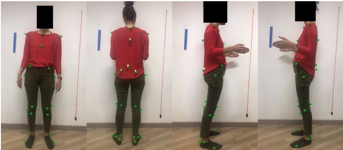
Figure B.55: Images captured with flash of the participant wearing a red shirt and green pants while using green styrofoam as markers. The markers detected by the software are surrounded with green circles. On the left: Anterior view. In the middle left: Posterior view. In the middle right: Right lateral view. On the right: Left lateral view.
