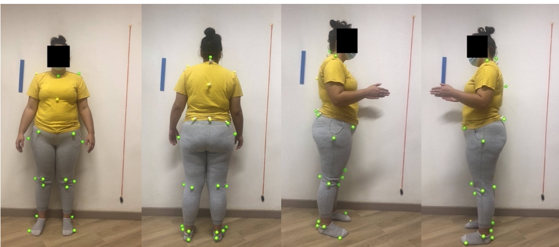
Figure B.20: Images captured without flash of the participant wearing a yellow shirt and gray pants while using yellow styrofoam spheres as markers. The markers detected by the software are surrounded with green circles. On the left: Anterior view. In the middle left: Posterior view. In the middle right: Right lateral view. On the right: Left lateral view.
