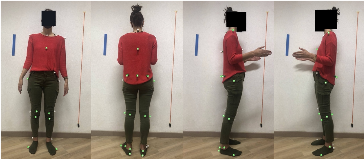
Figure B.16: Images captured without flash of the participant wearing a red shirt and green pants while using white styrofoam as markers. The markers detected by the software are surrounded with green circles. On the left: Anterior view. In the middle left: Posterior view. In the middle right: Right lateral view. On the right: Left lateral view.
