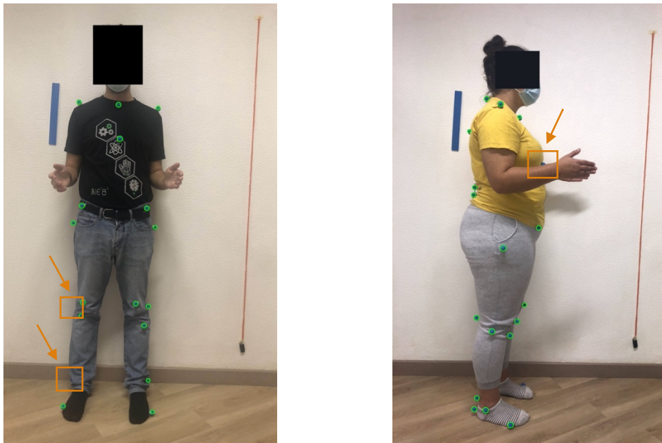
Figure 5.6: Images of the participants using blue styrofoam balls as markers, taken with a mobile phone camera. The green circles spot the detected area of the markers that were identified by the software. It demonstrates that when these markers are covered by body parts or by folds of the clothing, they are not detected by the software, which is identified with an orange box and arrow. On the left: Anterior view of the participant wearing a black shirt and jeans. On the right: Right lateral view of the participant wearing a yellow shirt and gray pants.
