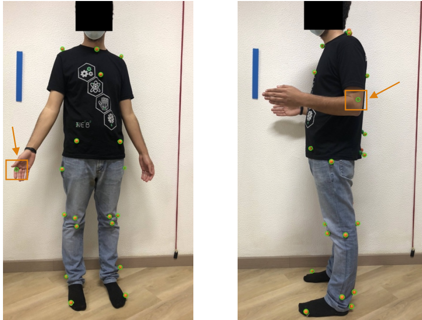
Figure 5.4: Images taken with a mobile phone camera without using flash of the participant wearing a black shirt and jeans, while using orange styrofoam balls as markers. The green circles spot the detected area of the markers that were identified by the software. It demonstrates the detection of false markers on the hands and arms of subjects due to the skin tone being inside the color threshold range, which are identified with an orange box and arrow. On the left: Anterior view. On the right: Left lateral view.
