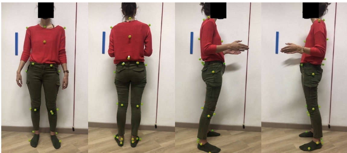
Figure B.32: Images captured without flash of the participant wearing a red shirt and green pants while using orange styrofoam as markers. The markers detected by the software are surrounded with green circles. On the left: Anterior view. In the middle left: Posterior view. In the middle right: Right lateral view. On the right: Left lateral view.
