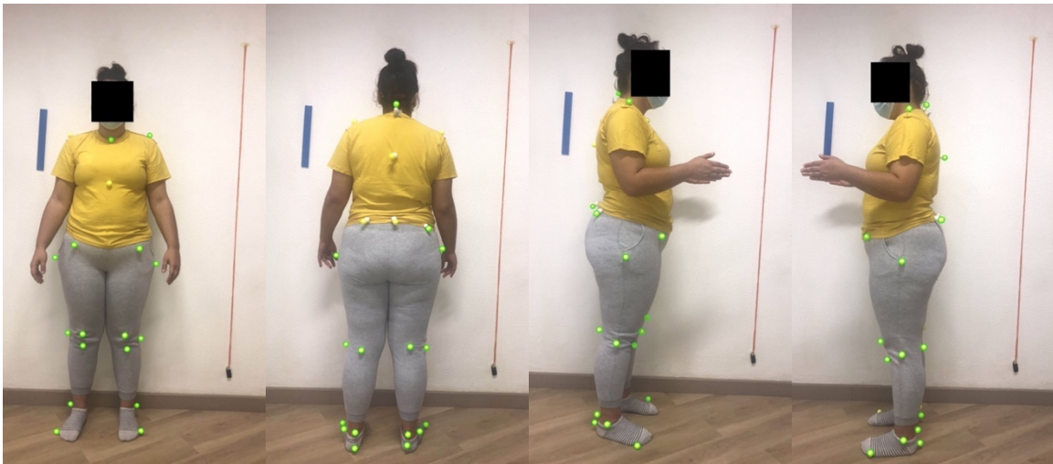
Figure B.19: Images captured with flash of the participant wearing a yellow shirt and gray pants while using yellow styrofoam spheres as markers. The markers detected by the software are surrounded with green circles. On the left: Anterior view. In the middle left: Posterior view. In the middle right: Right lateral view. On the right: Left lateral view.
