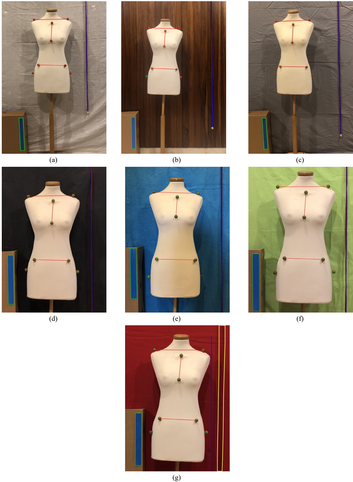
Figure 5.9: Images captured with a mobile phone camera without using flash. We varied the backgrounds of the images to understand the influence of their color on the detection of the markers, the blue rectangle, and the red string by our software. The detected markers are shown circled in red and are connected by red lines that represent the vectors used to calculate the angles. The blue rectangle is displayed with a green outline and the where the software considered the red string to be is represented by a dark blue line. In image (g) the true position of the red string is outlined in yellow. We tested as background the colors (a) white, (b) brown, (c) gray, (d) black, (e) blue, (f) green and (g) red.
