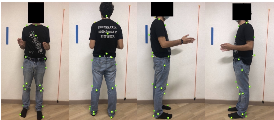
Figure B.17: Images captured with flash of the participant wearing a black shirt and jeans while using yellow styrofoam spheres as markers. The markers detected by the software are surrounded with green circles. On the left: Anterior view. In the middle left: Posterior view. In the middle right: Right lateral view. On the right: Left lateral view.
