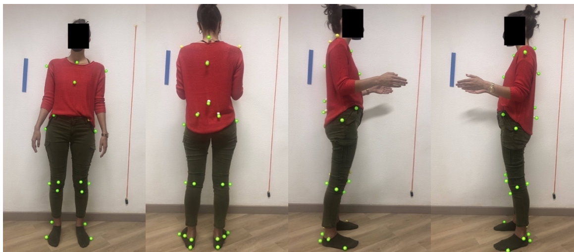
Figure B.23: Images captured with flash of the participant wearing a red shirt and green pants while using yellow styrofoam as markers. The markers detected by the software are surrounded with green circles. On the left: Anterior view. In the middle left: Posterior view. In the middle right: Right lateral view. On the right: Left lateral view.
