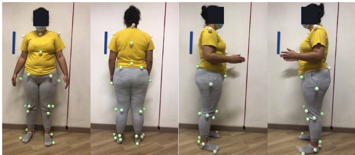
Figure B.4: Images captured without flash of the participant wearing a yellow shirt and gray pants while using white ping pong balls as markers. The markers detected by the software are surrounded with green circles. On the left: Anterior view. In the middle left: Posterior view. In the middle right: Right lateral view. On the right: Left lateral view.
