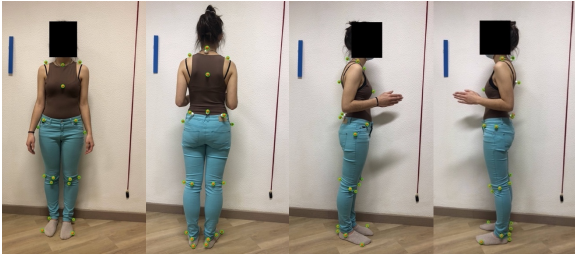
Figure B.30: Images captured without flash of the participant wearing a brown shirt and blue pants while using orange styrofoam spheres as markers. The markers detected by the software are surrounded with green circles. On the left: Anterior view. In the middle left: Posterior view. In the middle right: Right lateral view. On the right: Left lateral view.
