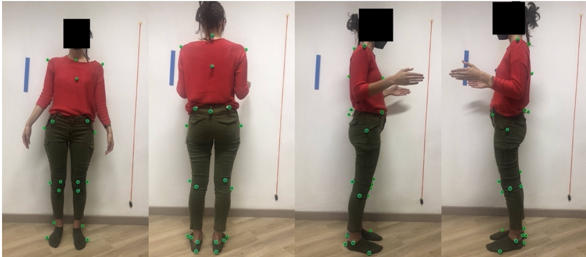
Figure B.48: Images captured without flash of the participant wearing a red shirt and green pants while using blue styrofoam as markers. The markers detected by the software are surrounded with green circles. On the left: Anterior view. In the middle left: Posterior view. In the middle right: Right lateral view. On the right: Left lateral view.
