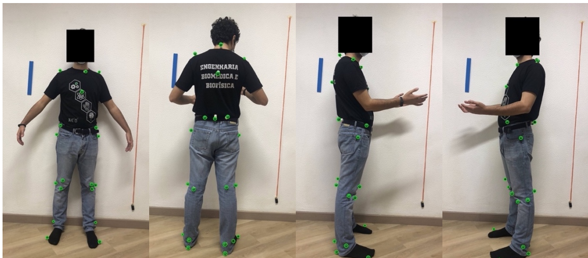
Figure B.50: Images captured without flash of the participant wearing a black shirt and jeans while using green styrofoam spheres as markers. The markers detected by the software are surrounded with green circles. On the left: Anterior view. In the middle left: Posterior view. In the middle right: Right lateral view. On the right: Left lateral view.
