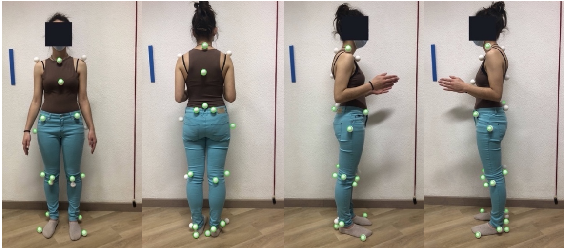
Figure B.6: Images captured without flash of the participant wearing a brown shirt and blue pants while using white ping pong balls as markers. The markers detected by the software are surrounded with green circles. On the left: Anterior view. In the middle left: Posterior view. In the middle right: Right lateral view. On the right: Left lateral view.
