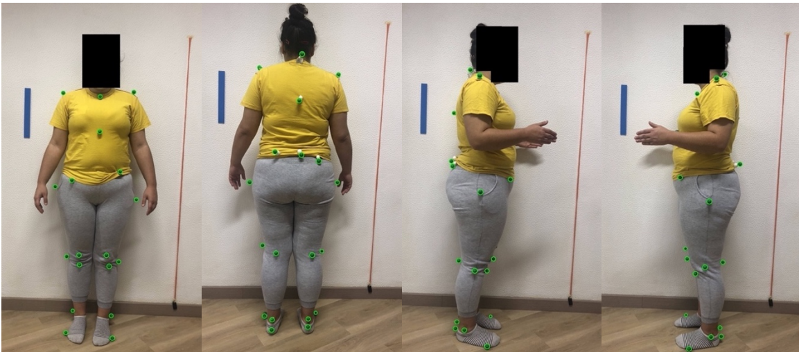
Figure B.52: Images captured with flash of the participant wearing a yellow shirt and gray pants while using green styrofoam spheres as markers. The markers detected by the software are surrounded with green circles. On the left: Anterior view. In the middle left: Posterior view. In the middle right: Right lateral view. On the right: Left lateral view.
