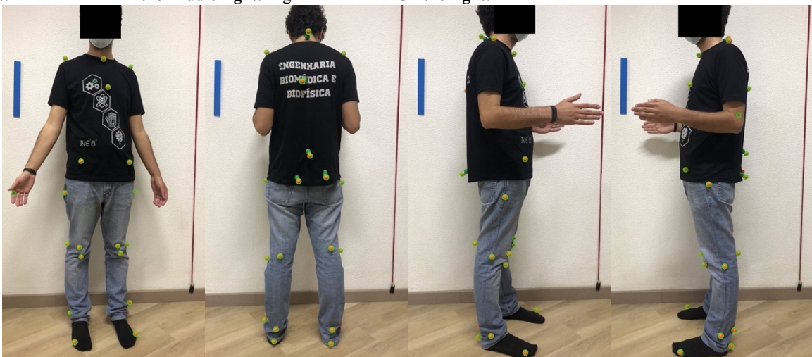
Figure B.26: Images captured without flash of the participant wearing a black shirt and jeans while using orange styrofoam spheres as markers. The markers detected by the software are surrounded with green circles. On the left: Anterior view. In the middle left: Posterior view. In the middle right: Right lateral view. On the right: Left lateral view.
