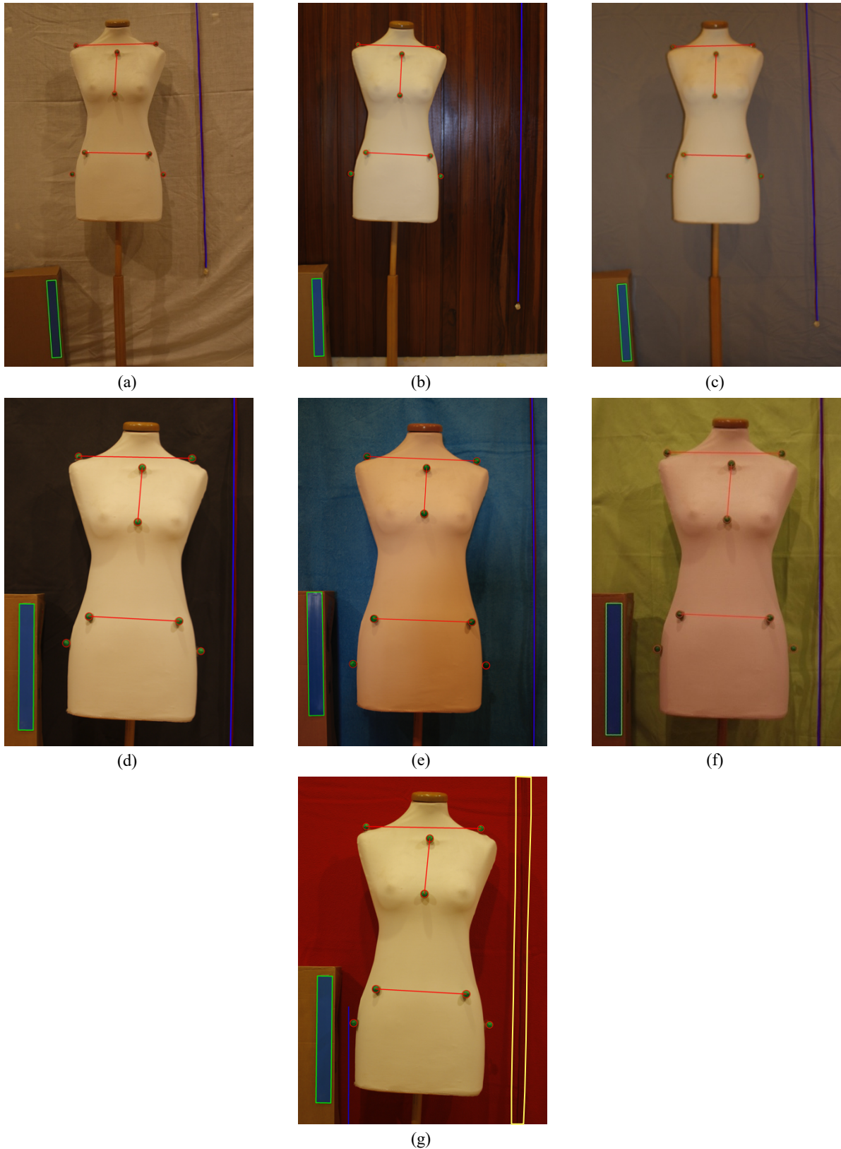
Figure 5.11: Images captured with a photographic camera without using flash. We varied the backgrounds of the images to understand the influence of their color on the detection of the markers, the blue rectangle, and the red string by our software. The detected markers are shown circled in red and are connected by red lines that represent the vectors used to calculate the angles. The blue rectangle is displayed with a green outline and the where the software considered the red string to be is represented by a dark blue line. In image (g) the true position of the red string is outlined in yellow. We tested as background the colors (a) white, (b) brown, (c) gray, (d) black, (e) blue, (f) green and (g) red.
