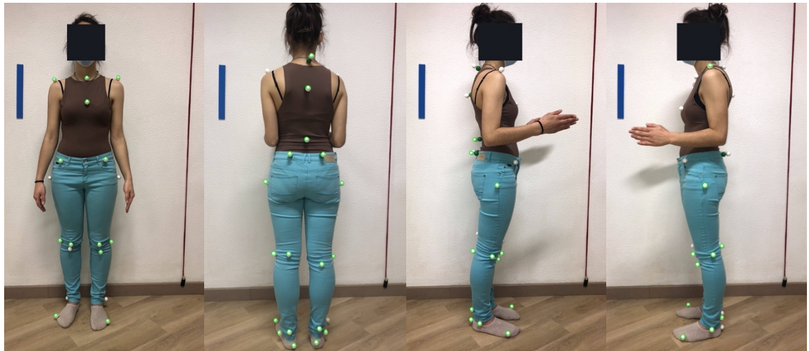
Figure B.13: Images captured with flash of the participant wearing a brown shirt and blue pants while using white styrofoam spheres as markers. The markers detected by the software are surrounded with green circles. On the left: Anterior view. In the middle left: Posterior view. In the middle right: Right lateral view. On the right: Left lateral view.
