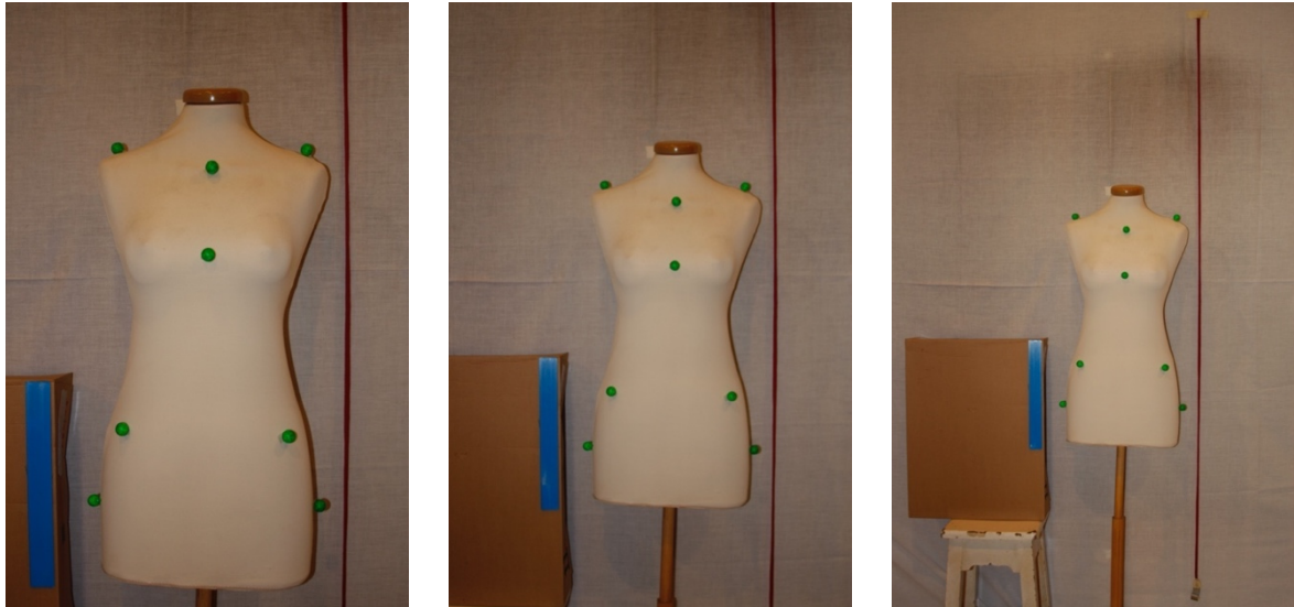
Figure C.7: Images captured using flash with a photographic camera at a height of 120 cm. We varied the distance of the camera to the markers. The camera is positioned on the left at 125 cm, in the middle at 180 cm and on the right at 250 cm.
