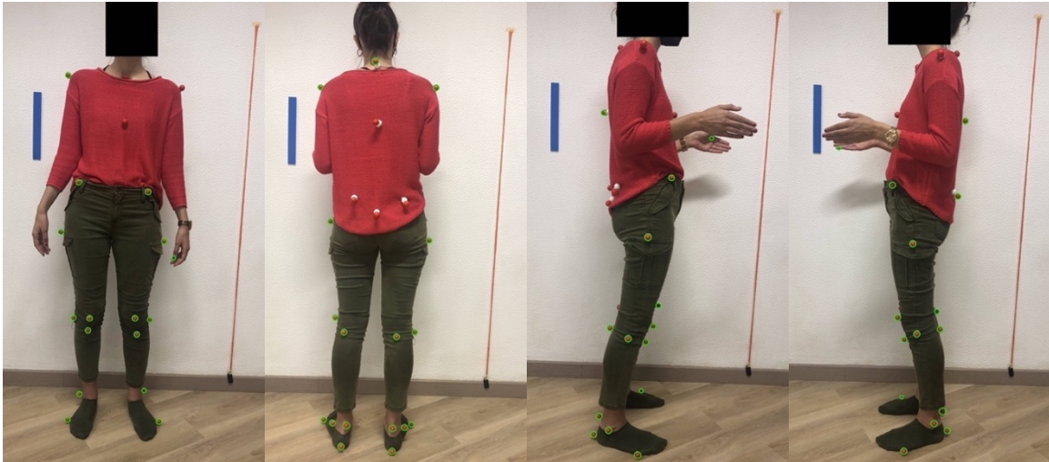
Figure B.39: Images captured with flash of the participant wearing a red shirt and green pants while using red styrofoam as markers. The markers detected by the software are surrounded with green circles. On the left: Anterior view. In the middle left: Posterior view. In the middle right: Right lateral view. On the right: Left lateral view.
