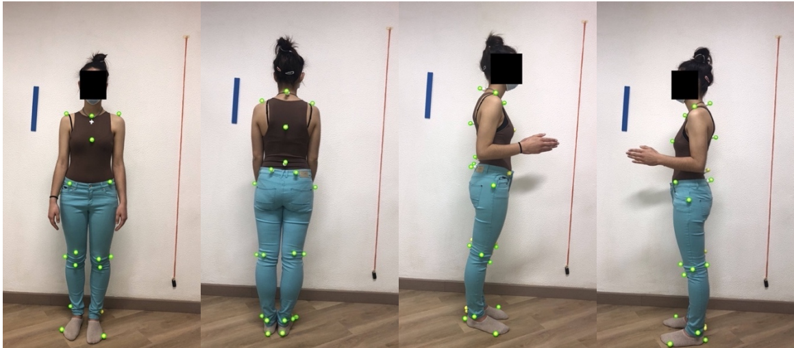
Figure B.21: Images captured with flash of the participant wearing a brown shirt and blue pants while using yellow styrofoam spheres as markers. The markers detected by the software are surrounded with green circles. On the left: Anterior view. In the middle left: Posterior view. In the middle right: Right lateral view. On the right: Left lateral view.
