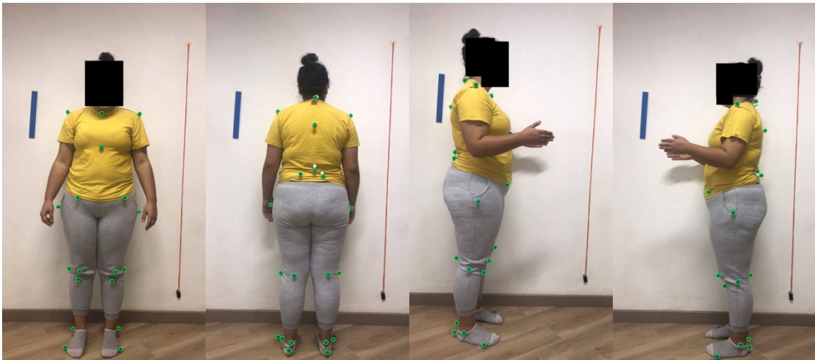
Figure B.43: Images captured with flash of the participant wearing a yellow shirt and gray pants while using blue styrofoam spheres as markers. The markers detected by the software are surrounded with green circles. On the left: Anterior view. In the middle left: Posterior view. In the middle right: Right lateral view. On the right: Left lateral view.
