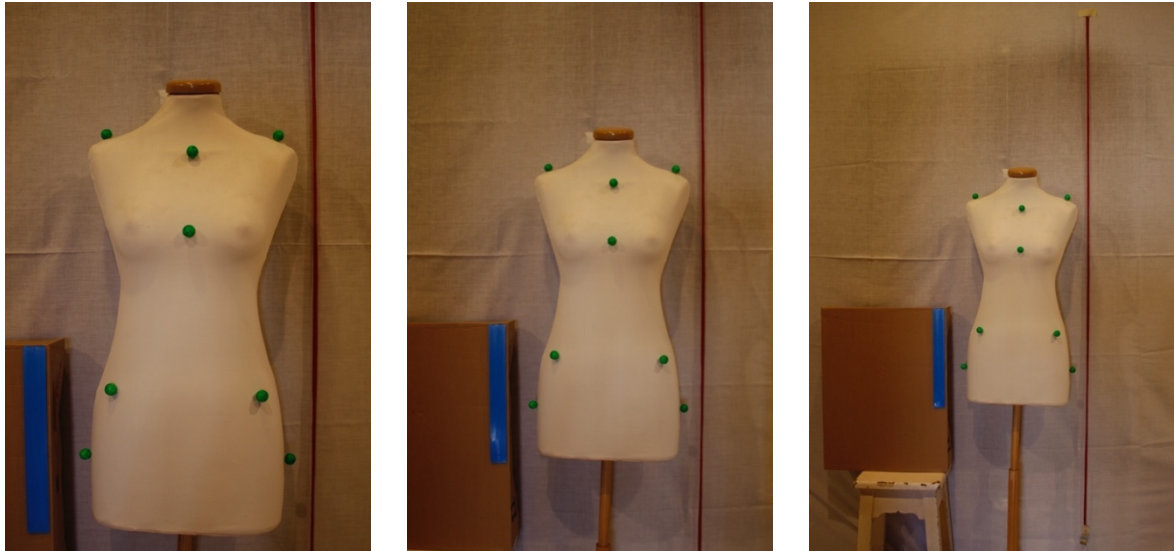
Figure C.10: Images captured without using flash with a photographic camera at a height of 120 cm. We varied the distance of the camera to the markers. The camera is positioned on the left at 125 cm, in the middle at 180 cm and on the right at 250 cm.
