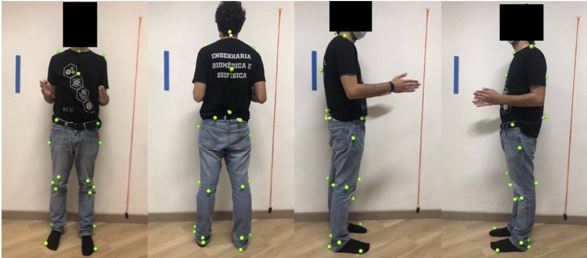
Figure B.18: Images captured without flash of the participant wearing a black shirt and jeans while using yellow styrofoam spheres as markers. The markers detected by the software are surrounded with green circles. On the left: Anterior view. In the middle left: Posterior view. In the middle right: Right lateral view. On the right: Left lateral view.
