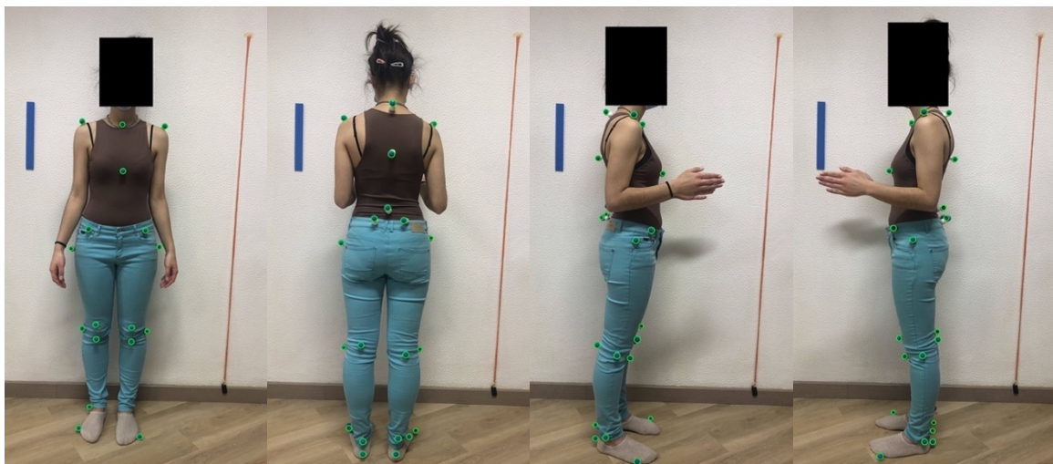
Figure B.46: Images captured without flash of the participant wearing a brown shirt and blue pants while using blue styrofoam spheres as markers. The markers detected by the software are surrounded with green circles. On the left: Anterior view. In the middle left: Posterior view. In the middle right: Right lateral view. On the right: Left lateral view.
