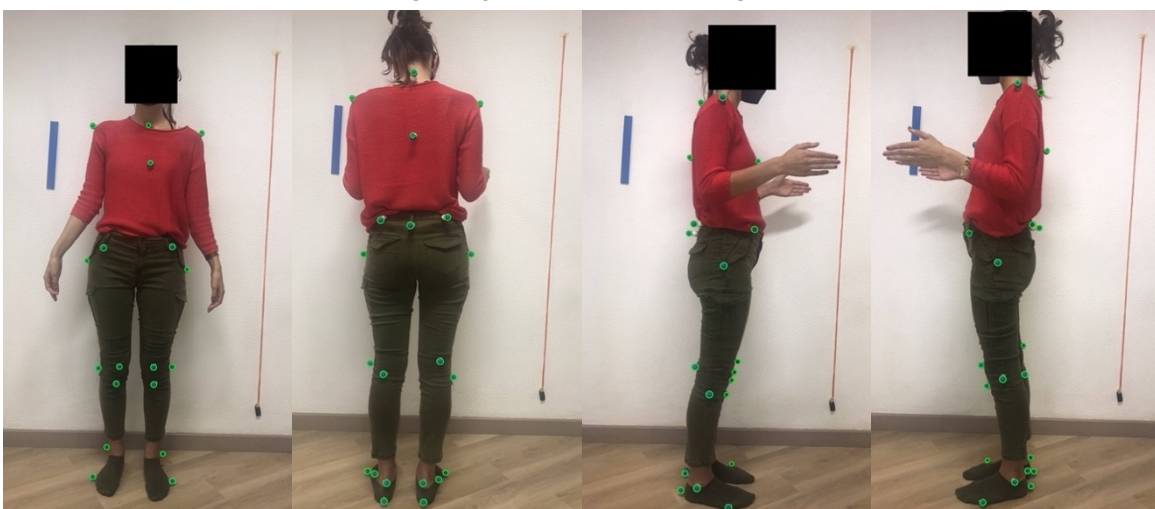
Figure B.47: Images captured with flash of the participant wearing a red shirt and green pants while using blue styrofoam as markers. The markers detected by the software are surrounded with green circles. On the left: Anterior view. In the middle left: Posterior view. In the middle right: Right lateral view. On the right: Left lateral view.
