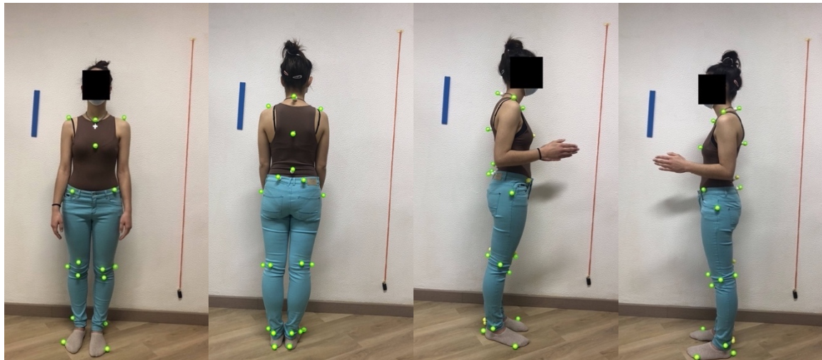
Figure B.22: Images captured without flash of the participant wearing a brown shirt and blue pants while using yellow styrofoam spheres as markers. The markers detected by the software are surrounded with green circles. On the left: Anterior view. In the middle left: Posterior view. In the middle right: Right lateral view. On the right: Left lateral view.
