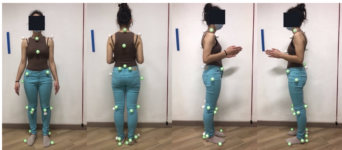
Figure B.5: Images captured with flash of the participant wearing a brown shirt and blue pants while using white ping pong balls as markers. The markers detected by the software are surrounded with green circles. On the left: Anterior view. In the middle left: Posterior view. In the middle right: Right lateral view. On the right: Left lateral view.
