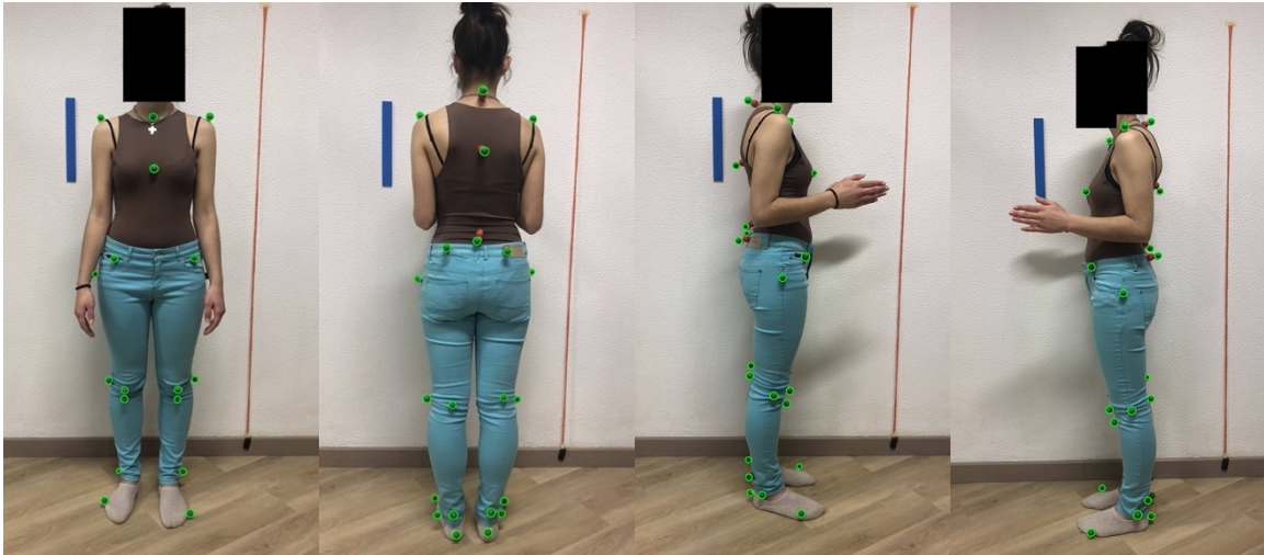
Figure B.54: Images captured without flash of the participant wearing a brown shirt and blue pants while using green styrofoam spheres as markers. The markers detected by the software are surrounded with green circles. On the left: Anterior view. In the middle left: Posterior view. In the middle right: Right lateral view. On the right: Left lateral view.
