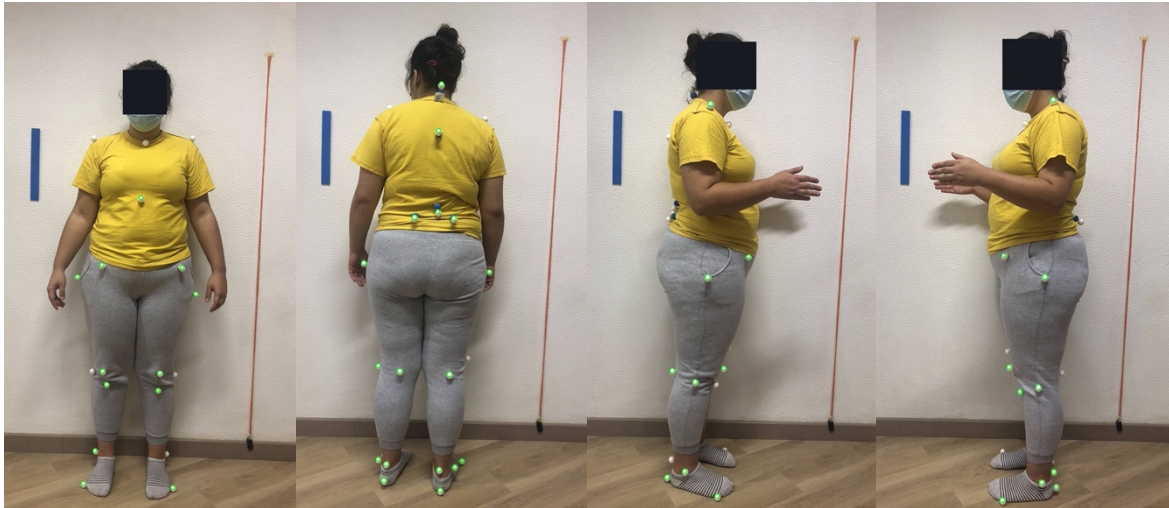
Figure B.12: Images captured without flash of the participant wearing a yellow shirt and gray pants while using white styrofoam spheres as markers. The markers detected by the software are surrounded with green circles. On the left: Anterior view. In the middle left: Posterior view. In the middle right: Right lateral view. On the right: Left lateral view.
