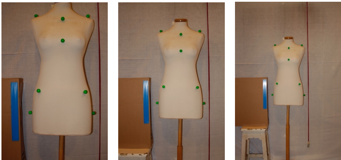
Figure C.9: Images captured using flash with a photographic camera at a height of 100 cm. We varied the distance of the camera to the markers. The camera is positioned on the left at 125 cm, in the middle at 180 cm and on the right at 250 cm.
