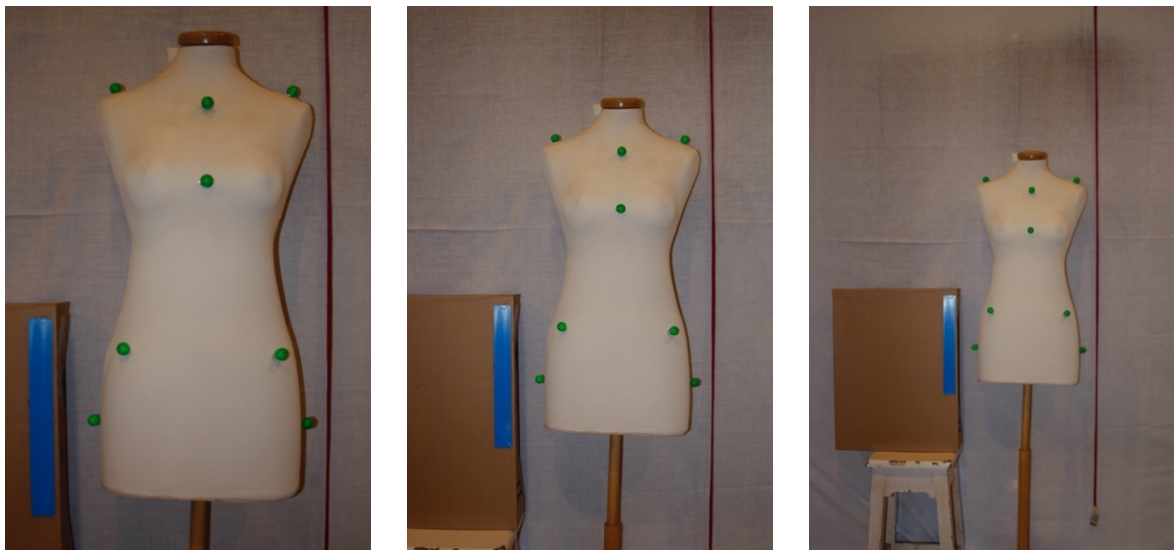
Figure C.8: Images captured using flash with a photographic camera at a height of 110 cm. We varied the distance of the camera to the markers. The camera is positioned on the left at 125 cm, in the middle at 180 cm and on the right at 250 cm.
