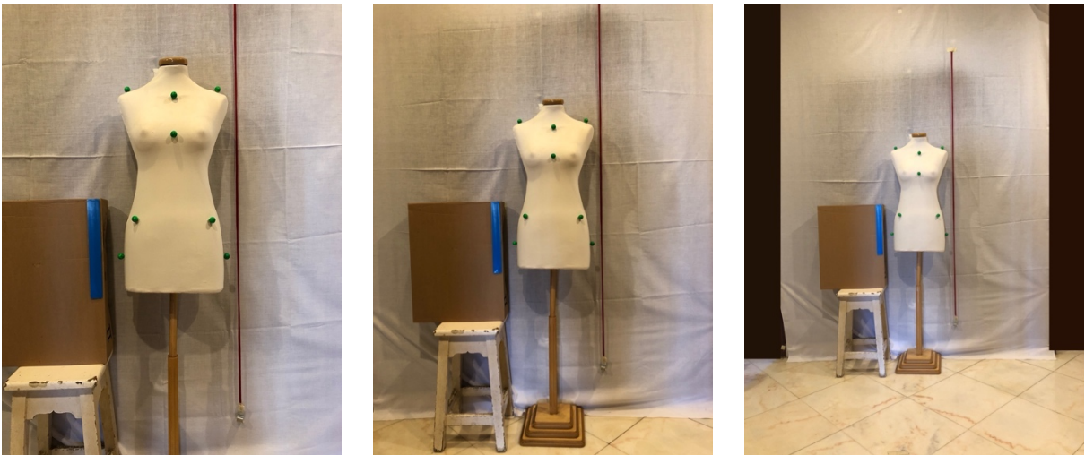
Figure C.6: Images captured without using flash with a mobile phone camera at a height of 100 cm. We varied the distance of the camera to the markers. The camera is positioned on the left at 125 cm, in the middle at 180 cm and on the right at 250 cm.
