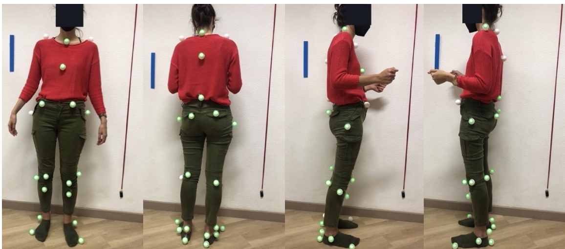
Figure B.8: Images captured without flash of the participant wearing a red shirt and green pants while using white ping pong balls as markers. The markers detected by the software are surrounded with green circles. On the left: Anterior view. In the middle left: Posterior view. In the middle right: Right lateral view. On the right: Left lateral view.
