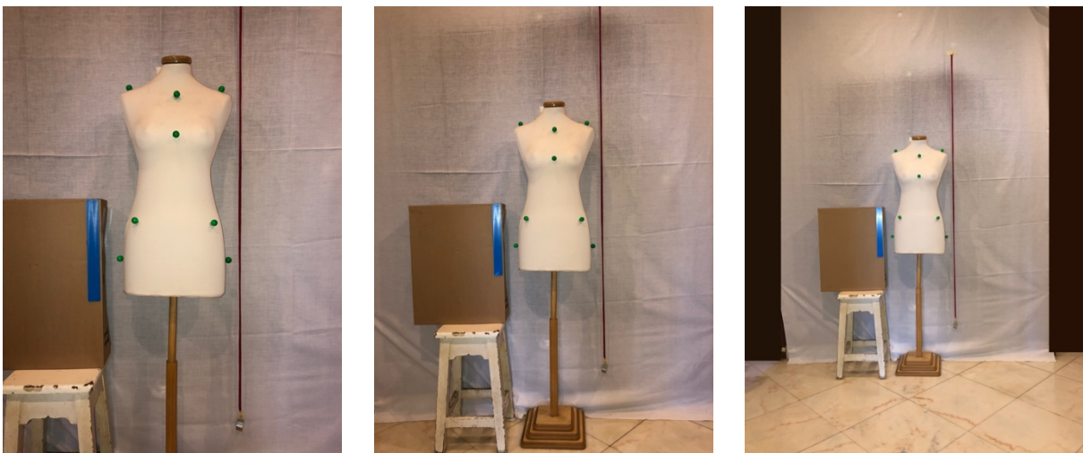
Figure C.3: Images captured using flash with a mobile phone camera at a height of 100 cm. We varied the distance of the camera to the markers. The camera is positioned on the left at 125 cm, in the middle at 180 cm and on the right at 250 cm.
