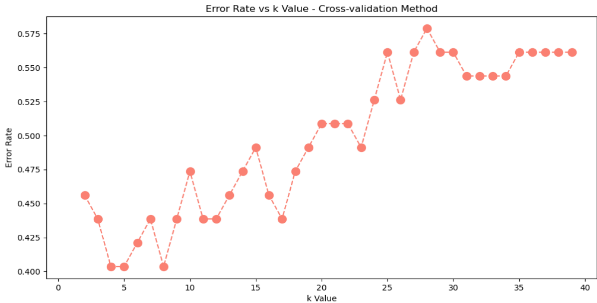
Figure 5.26: Graph of the error rate variation in function of k value when implementing the kNN algorithm with the cross-validation method to classify the subjects into the three classes: “without evidence”, “with mild evidence” and “with moderate to severe evidence”. The five k values that correspond to the first five lowest error rates are k=4, k=5, k=6, k=8 and k=12.
