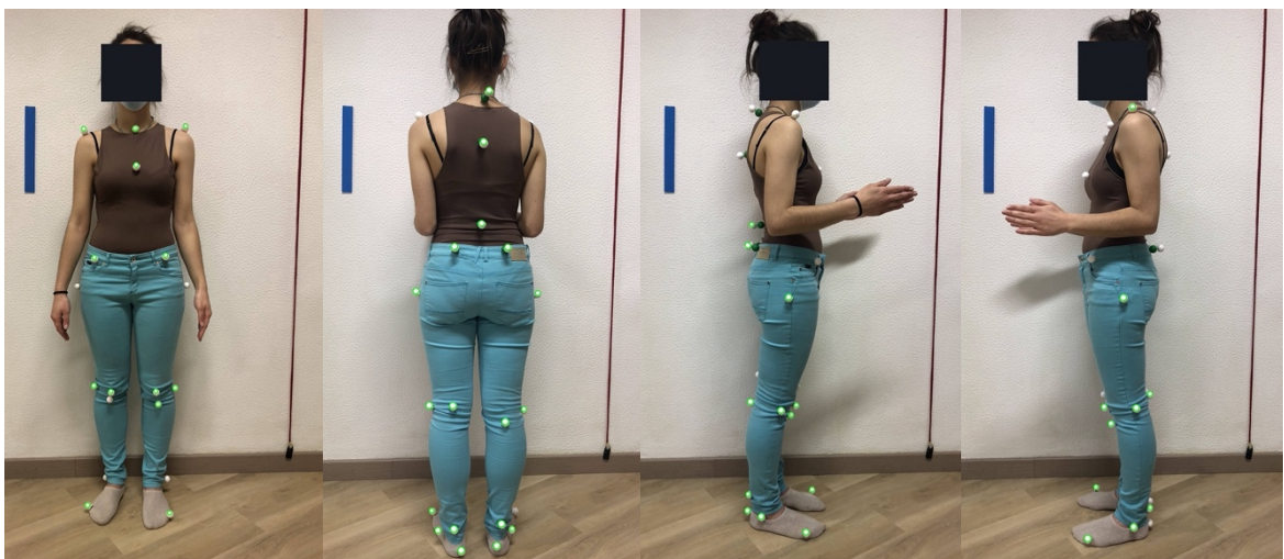
Figure B.14: Images captured without flash of the participant wearing a brown shirt and blue pants while using white styrofoam spheres as markers. The markers detected by the software are surrounded with green circles. On the left: Anterior view. In the middle left: Posterior view. In the middle right: Right lateral view. On the right: Left lateral view.
