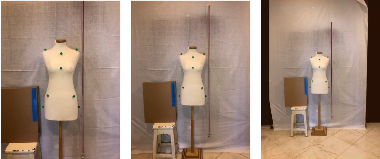
Figure C.1: Images captured using flash with a mobile phone camera at a height of 120 cm. We varied the distance of the camera to the markers. The camera is positioned on the left at 125 cm, in the middle at 180 cm and on the right at 250 cm.
