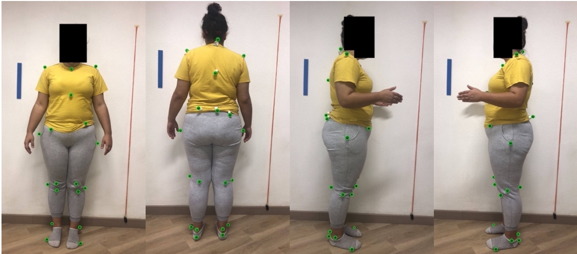
Figure B.51: Images captured with flash of the participant wearing a yellow shirt and gray pants while using green styrofoam spheres as markers. The markers detected by the software are surrounded with green circles. On the left: Anterior view. In the middle left: Posterior view. In the middle right: Right lateral view. On the right: Left lateral view.
