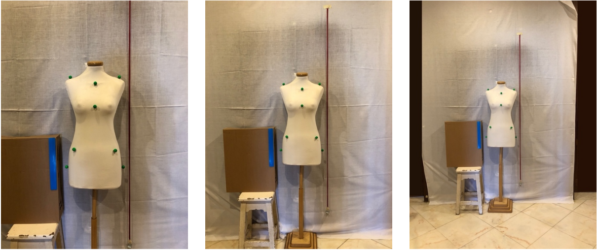
Figure C.4: Images captured without using flash with a mobile phone camera at a height of 120 cm. We varied the distance of the camera to the markers. The camera is positioned on the left at 125 cm, in the middle at 180 cm and on the right at 250 cm.
