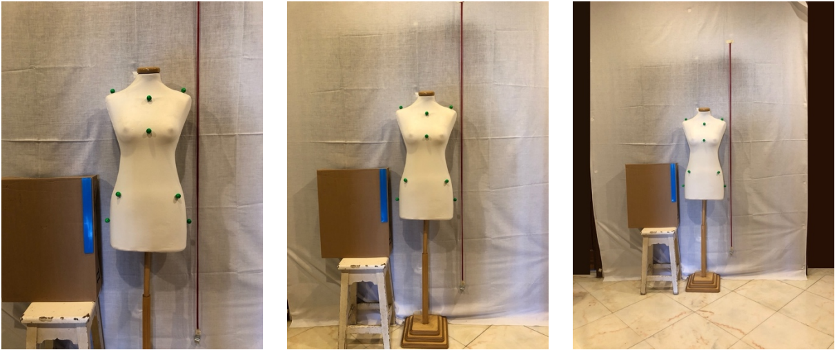
Figure C.5: Images captured without using flash with a mobile phone camera at a height of 110 cm. We varied the distance of the camera to the markers. The camera is positioned on the left at 125 cm, in the middle at 180 cm and on the right at 250 cm.
