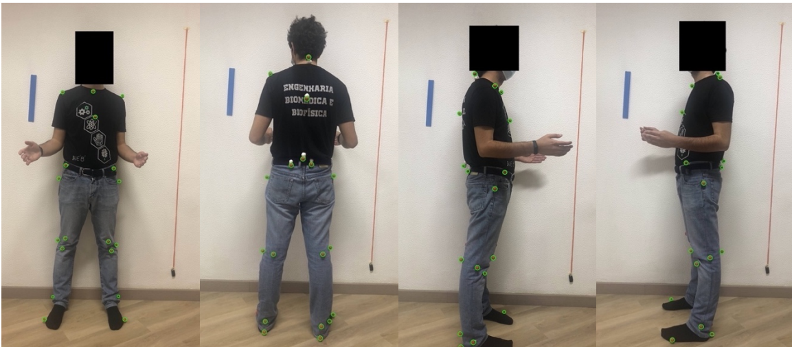
Figure B.34: Images captured without flash of the participant wearing a black shirt and jeans while using red styrofoam spheres as markers. The markers detected by the software are surrounded with green circles. On the left: Anterior view. In the middle left: Posterior view. In the middle right: Right lateral view. On the right: Left lateral view.
