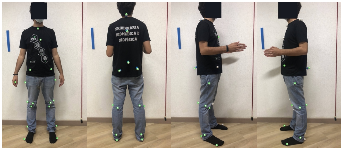
Figure B.10: Images captured without flash of the participant wearing a black shirt and jeans while using white styrofoam spheres as markers. The markers detected by the software are surrounded with green circles. On the left: Anterior view. In the middle left: Posterior view. In the middle right: Right lateral view. On the right: Left lateral view.
