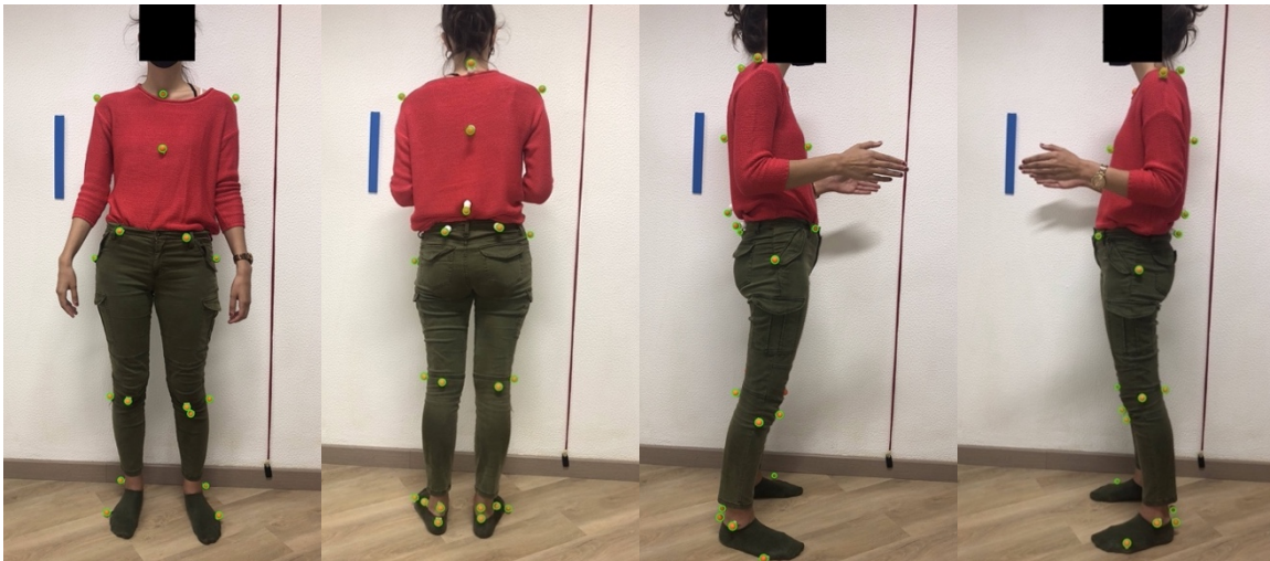
Figure B.31: Images captured with flash of the participant wearing a red shirt and green pants while using orange styrofoam as markers. The markers detected by the software are surrounded with green circles. On the left: Anterior view. In the middle left: Posterior view. In the middle right: Right lateral view. On the right: Left lateral view.
