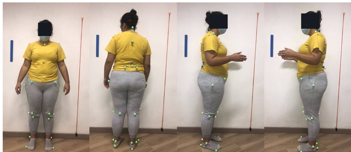
Figure B.11: Images captured with flash of the participant wearing a yellow shirt and gray pants while using white styrofoam spheres as markers. The markers detected by the software are surrounded with green circles. On the left: Anterior view. In the middle left: Posterior view. In the middle right: Right lateral view. On the right: Left lateral view.
