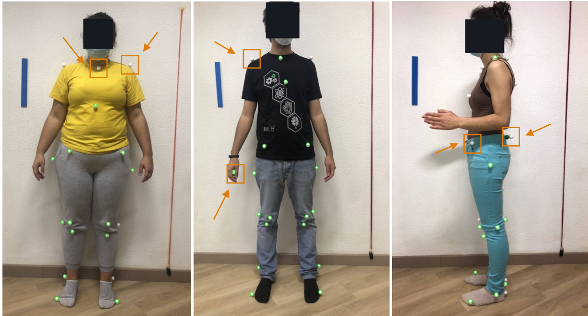
Figure 5.2: Images of the participants using white styrofoam balls as markers, taken with a mobile phone camera. The green circles spot the detected area of the markers that were identified by the software. It demonstrates that when these markers have a white wall as a background or when they have shadows caused by body parts, they are not fully distinguished by the software. Also, it shows the detection of false markers due to similar color between the background and the markers. These situations are identified with an orange box and arrow. On the left: Anterior view of the participant wearing a yellow shirt and gray pants. In the middle: Anterior view of the participant wearing a black shirt and jeans. On the right: Left lateral view of the participant wearing a brown shirt and blue pants.
