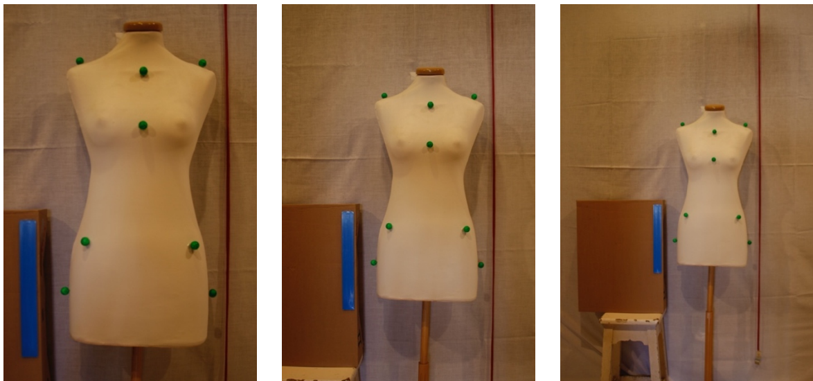
Figure C.11: Images captured without using flash with a photographic camera at a height of 110 cm. We varied the distance of the camera to the markers. The camera is positioned on the left at 125 cm, in the middle at 180 cm and on the right at 250 cm.
