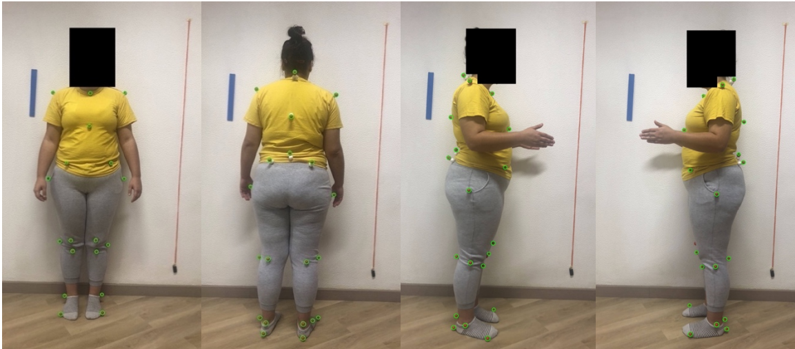
Figure B.36: Images captured without flash of the participant wearing a yellow shirt and gray pants while using red styrofoam spheres as markers. The markers detected by the software are surrounded with green circles. On the left: Anterior view. In the middle left: Posterior view. In the middle right: Right lateral view. On the right: Left lateral view.
