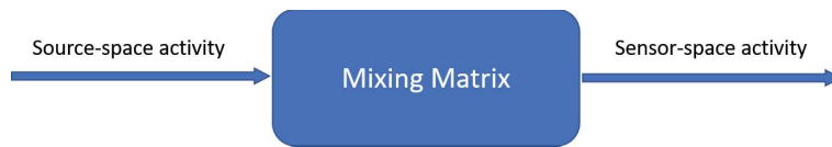
Figure 4.5: Representation of a simple linear forward model with EEG electrode activity as the model's response
