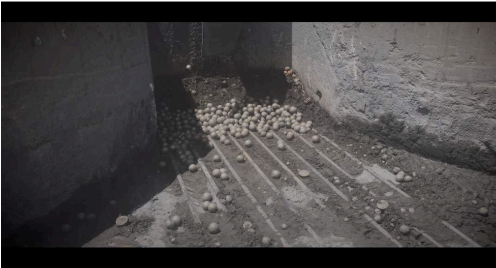
Steel grinding balls used to extract the ore from the waste rock. Still from the film Withering Refuge , Pedro F. Neto 2020
