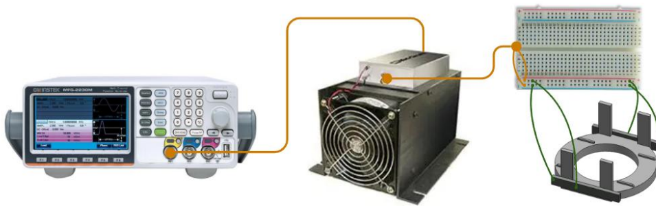
Figure 2.5 - Scheme of the acoustic manipulation circuit. Composed by a signal generator, a voltage amplifier, a breadboard and a setup (A, B, C or D). Setup B is illustrated as an example.
