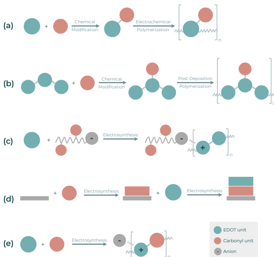
Figure 1.7 – Representation of the most common strategies to synthesize hybrid carbonyl and PEDOT-based materials.
